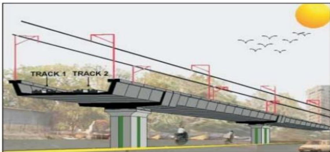
Fig.2.13 U-Girder (Precast Segmental) Supporting 2 Tracks
