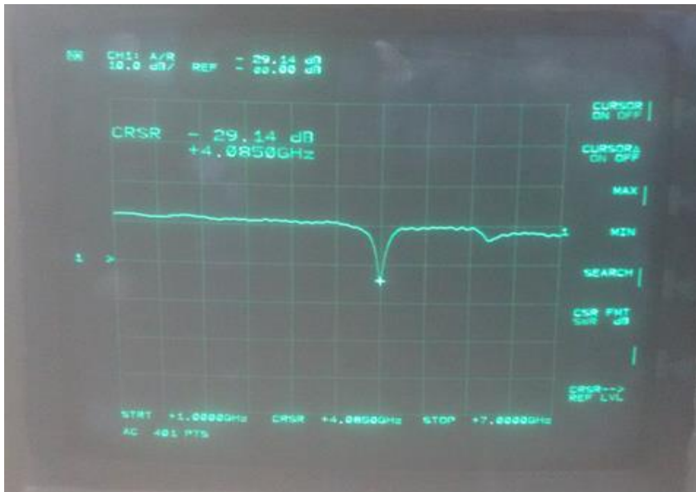
Fig. 3.43: Tested result of the CSRR loaded patch antenna on network analyzer.
