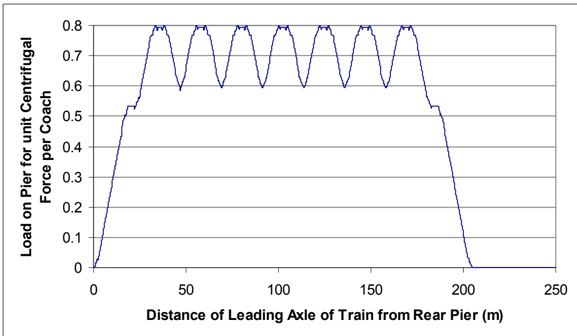
Fig. 4.9 Centrifugal Force on Pier for Different Train Placements on 16 m span
