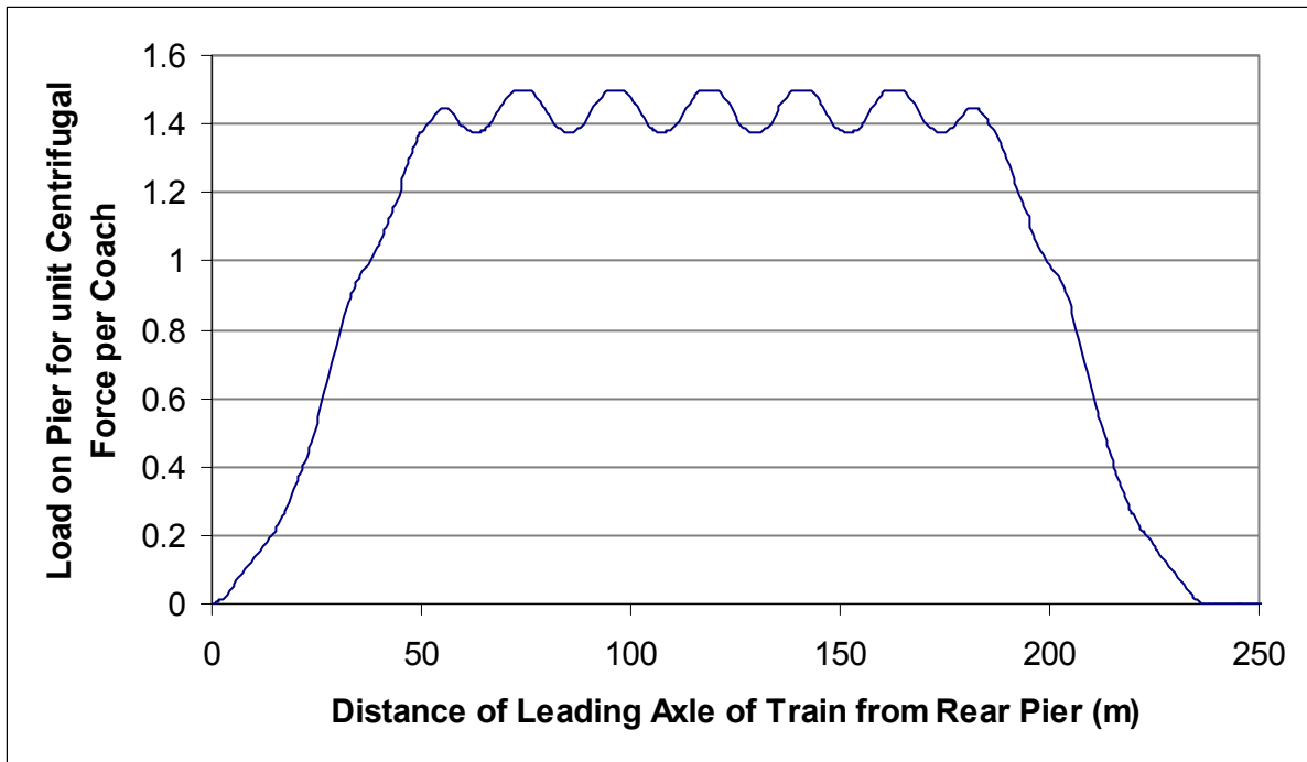
Fig. 4.17 Centrifugal Force on Pier for Different Train Placements on 32 m span
