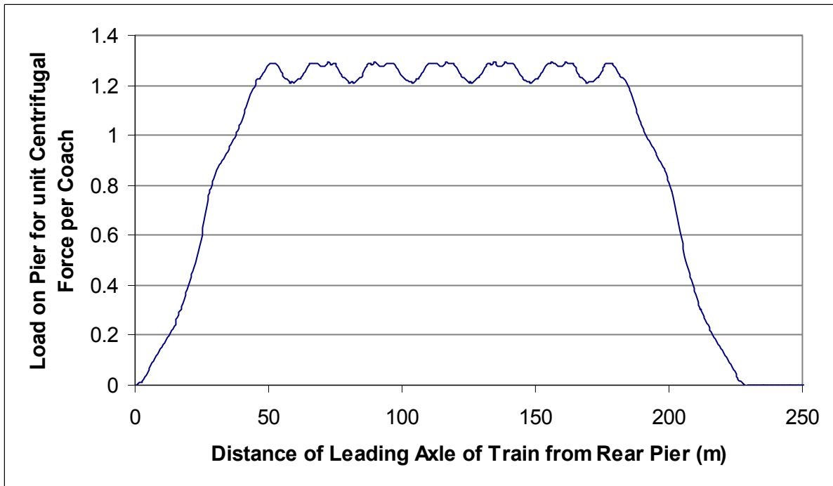
Fig. 4.15 Centrifugal Force on Pier for Different Train Placements on 28 m span
