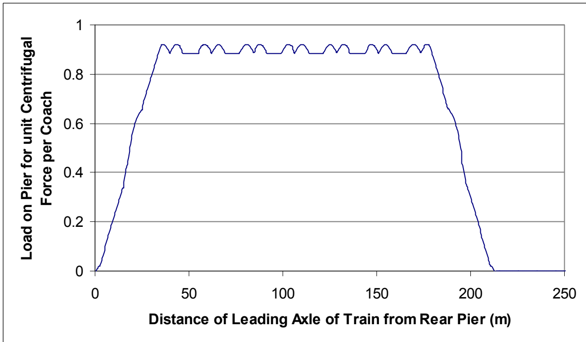
Fig. 4.11 Centrifugal Force on Pier for Different Train Placements on 20 m span
