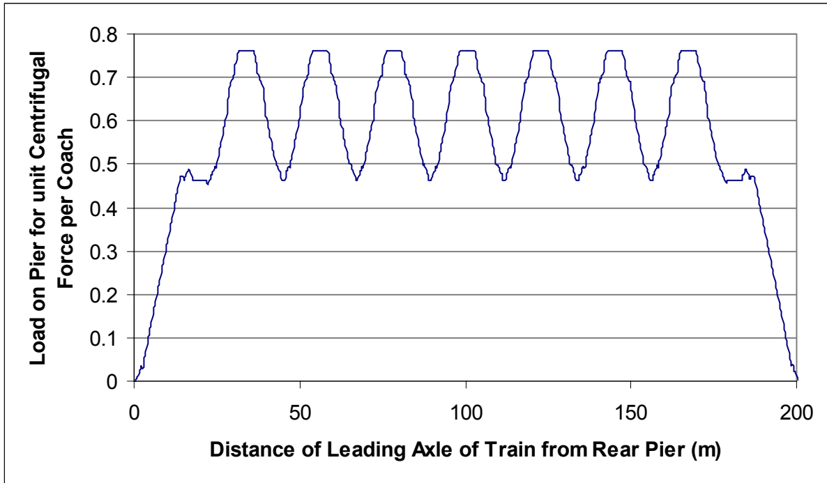
Fig. 4.8 Centrifugal Force on Pier for Different Train Placements on 14 m span
