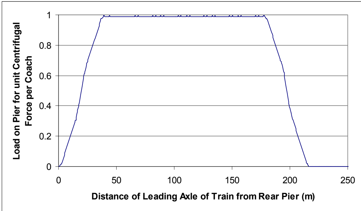
Fig. 4.12 Centrifugal Force on Pier for Different Train Placements on 22 m span
