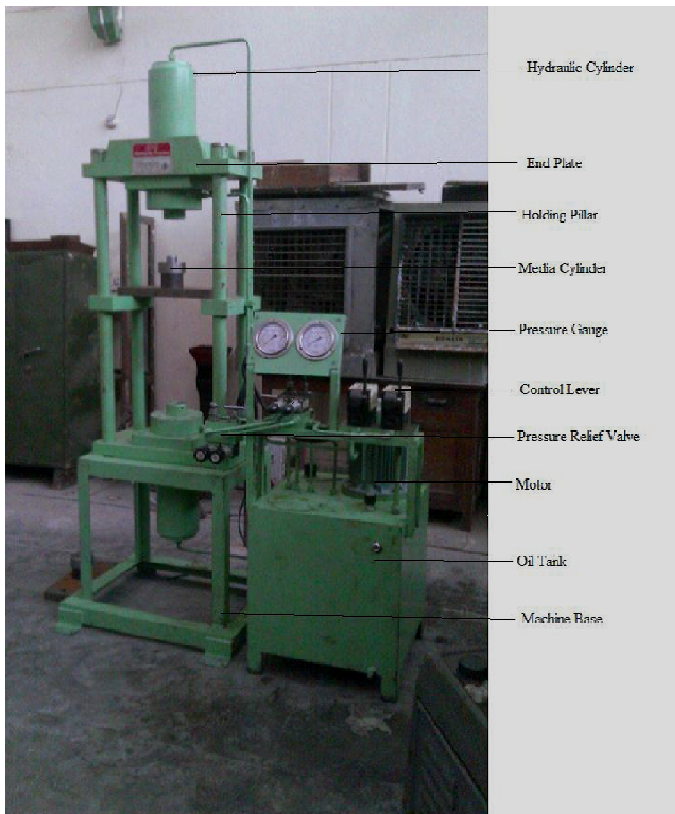
Figure 6. Vertical double acting AFM machine setup
