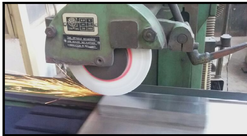
Figure 3.13: Grinding process on workpiece
