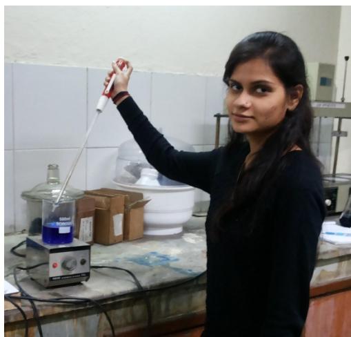
Figure 3.5: Methylene Blue Desorption experimental set up using Magnetic Stirrer
