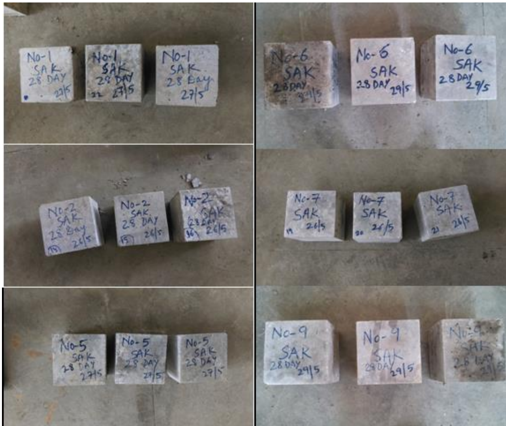
Fig 3.9 Concrete cubes with different sludge and flyash contents as per L9 Orthogonal Array
