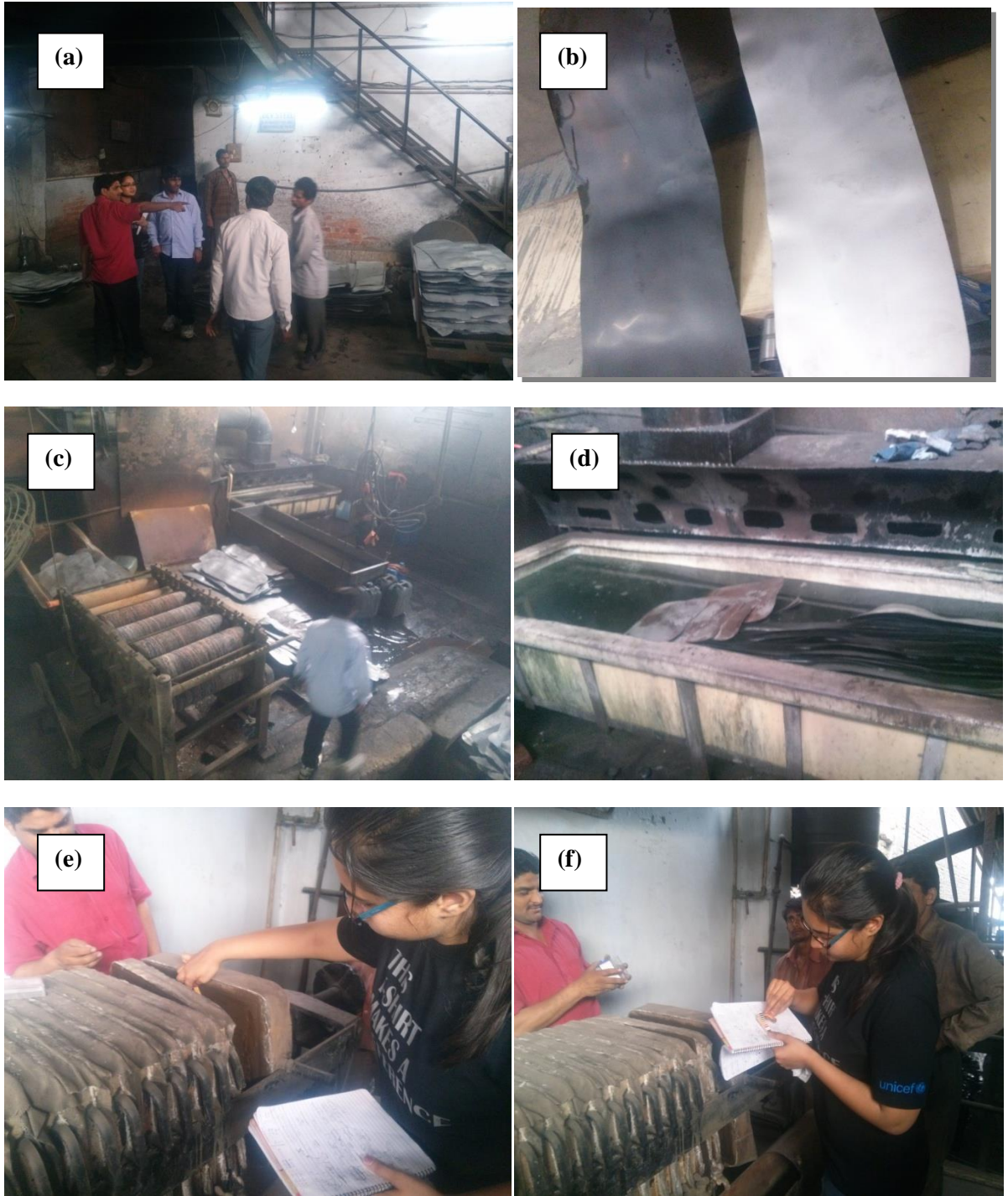
Fig 3.1 Industrial Visit to the Stainless Steel Pickling Industry in Wazirpur Industrial Area. (a) Industry premises, (b) Stainless steel sheet before and after pickling, (c) Pickling Line, (d) Pickling bath, (e) Filter press of ETP and (f) Field analysis of pH of sludge using filter paper.
