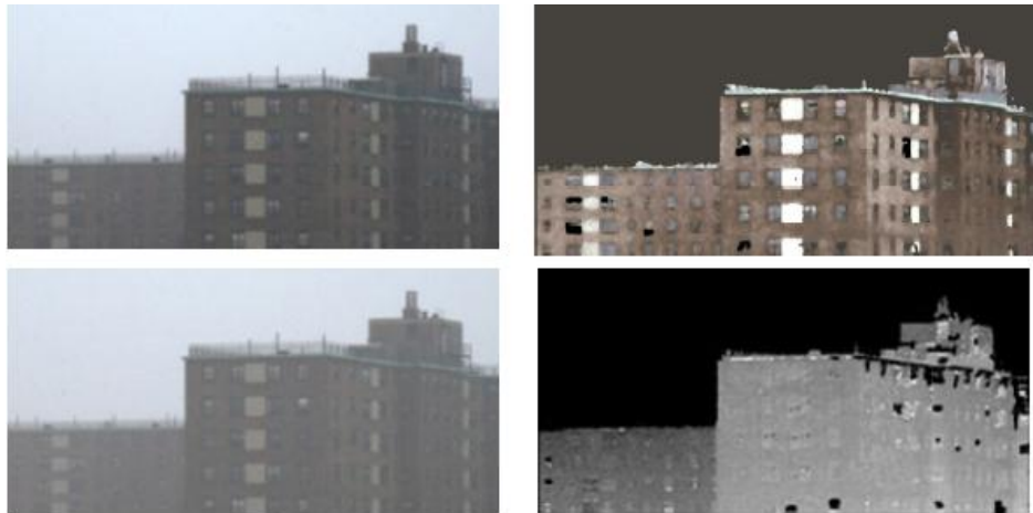
Figure 2.8: Haze removal based on varying atmospheric conditions. On the left are two images taken in two hazy conditions. On the right are the estimated image and depth (the sky is ignored).
