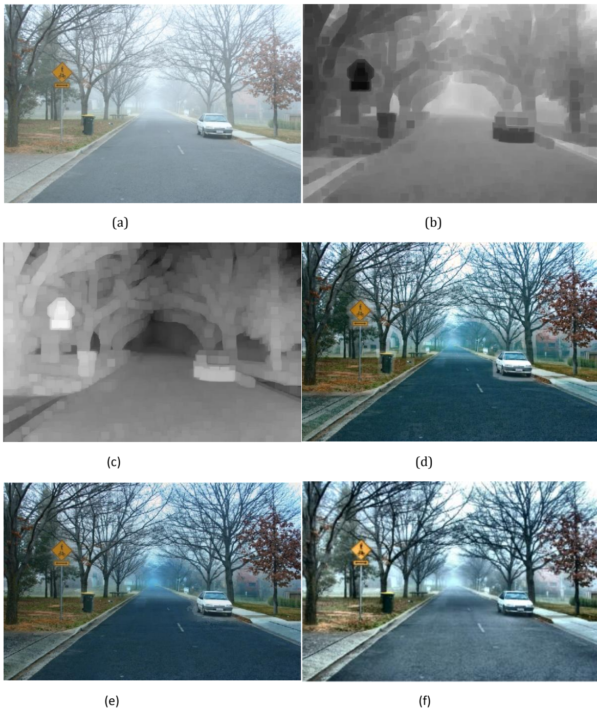
Fig. 6.1. Scene radiance recovery using different filtering radii r (patch size of dark channel is 15 \times 15 , \epsilon = 10^{-3} ). (a) Input hazy image. (b) Dark channel. (c) Coarse transmission map. (d)(e)(f) Scene radiance recovered with r equals to 8, 80, and 800, respectively.
