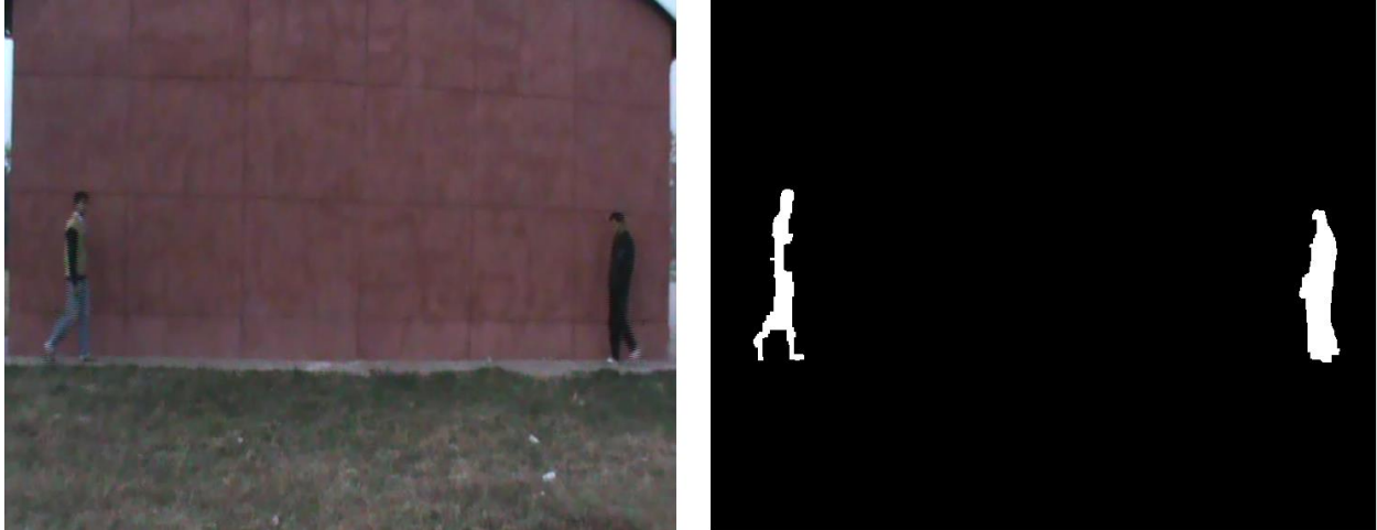
Fig 2.1 Foreground detected after background subtraction using GMM
