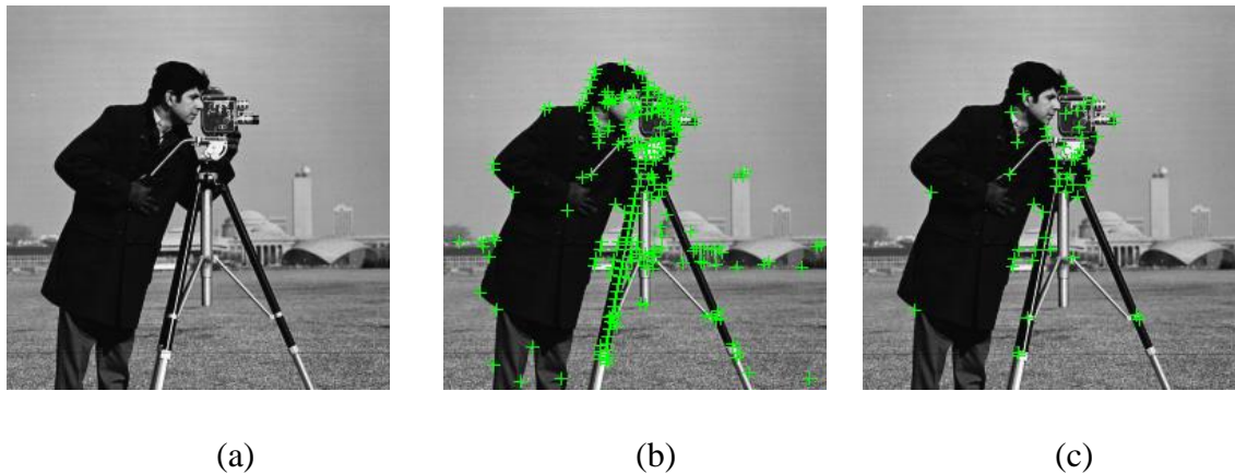
Fig 4.3 Detection of FAST Features. (a) Original image, (b) FAST features extracted, (c) strongest 50 FAST features
