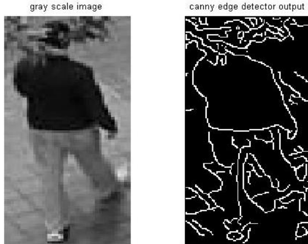
Fig 3.4 Canny edge detector output of object's image in frame
