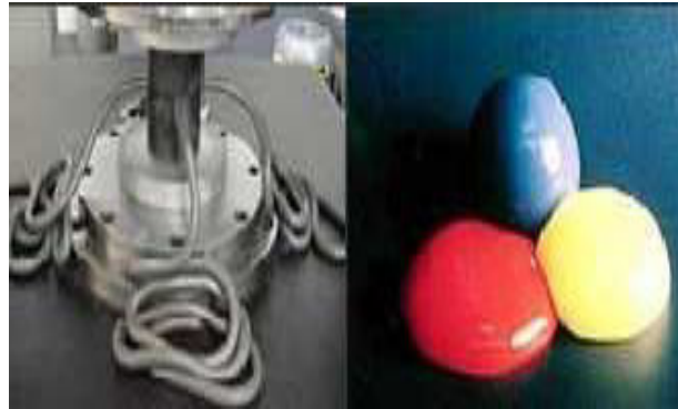
Fig 5. Extrude Hone's abrasive media [16]
