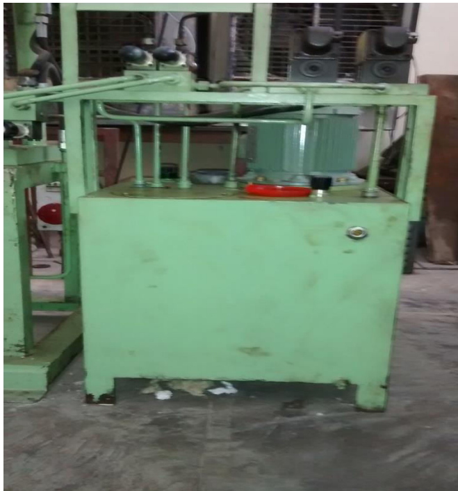
Fig. 7 Photograph of Hydraulic power pack
