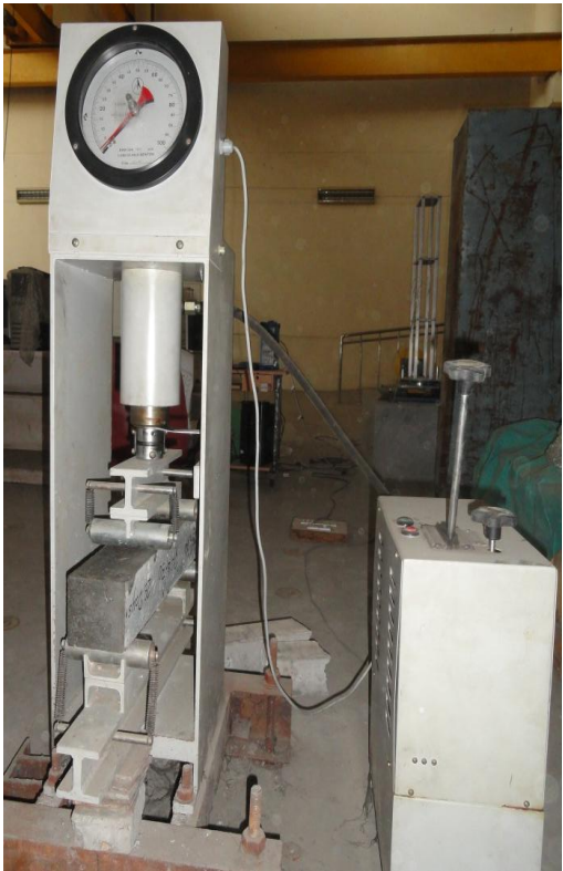
Figure 5.2: Photo showing flexural test of beam specimen
