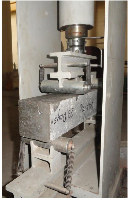
Figure 5.2: Photo showing flexural test of beam specimen
