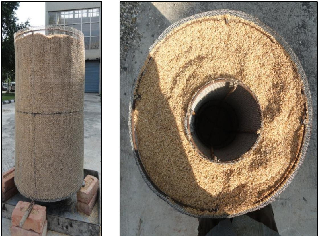
Figure 3.4 Elevation and top view of Burner after being filled by rice husk
