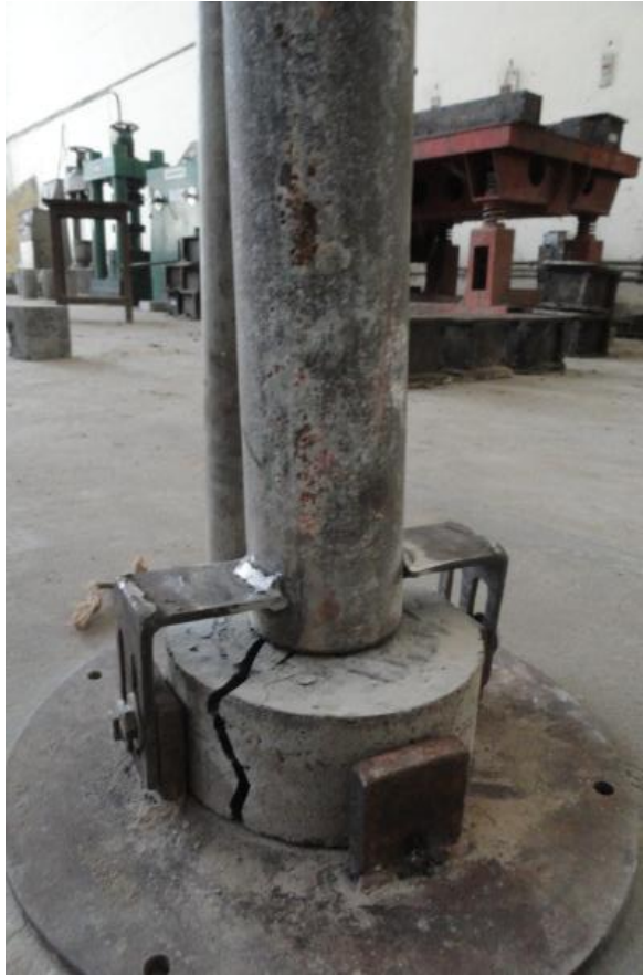
Figure 4.19: Photo of failed specimen
