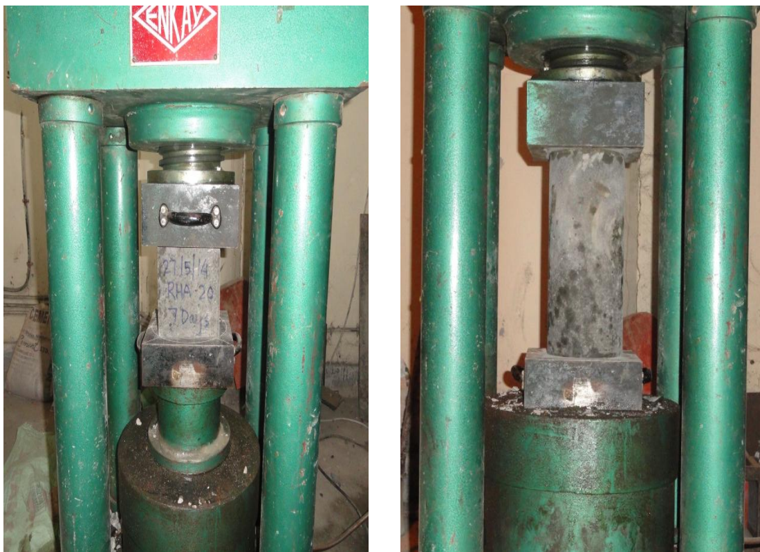
Figure 5.1: Photo showing compressive test of cubes and cylinder specimens
