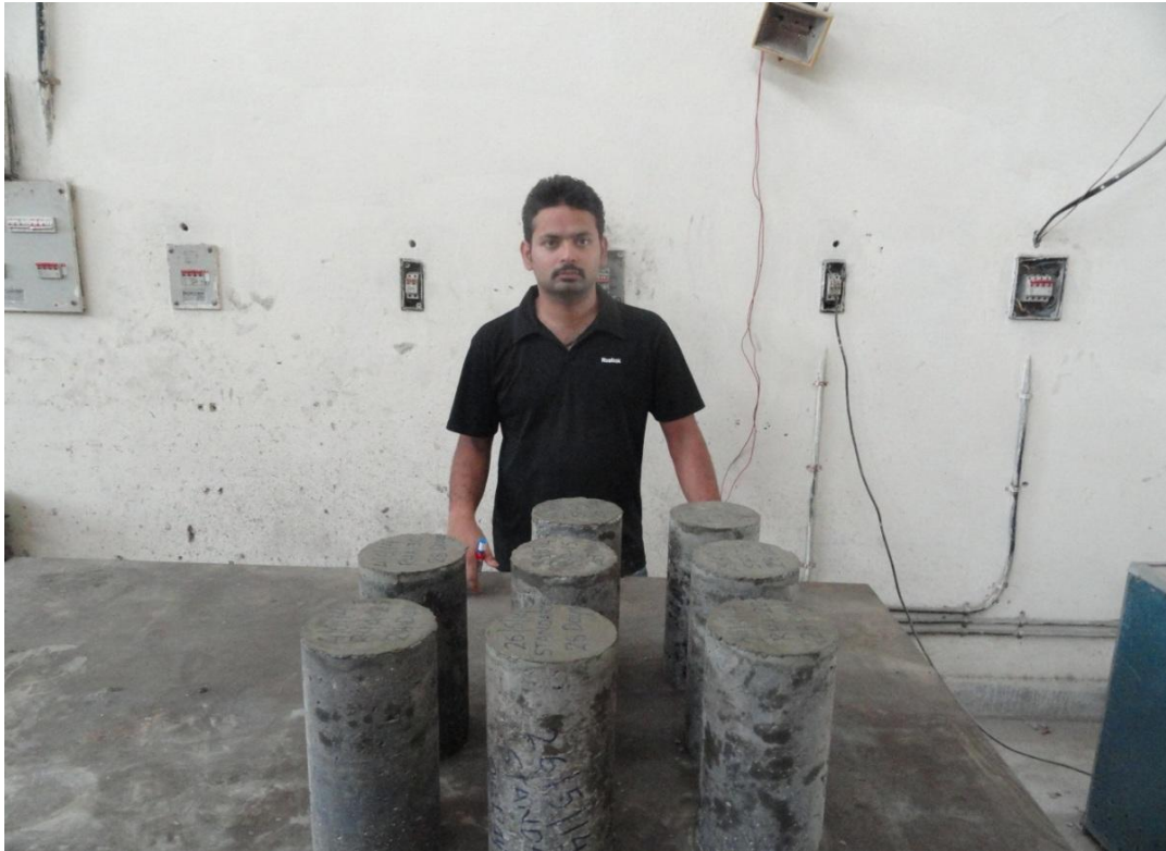
Figure 4.11: Photo of cylinders for testing at 90 days
