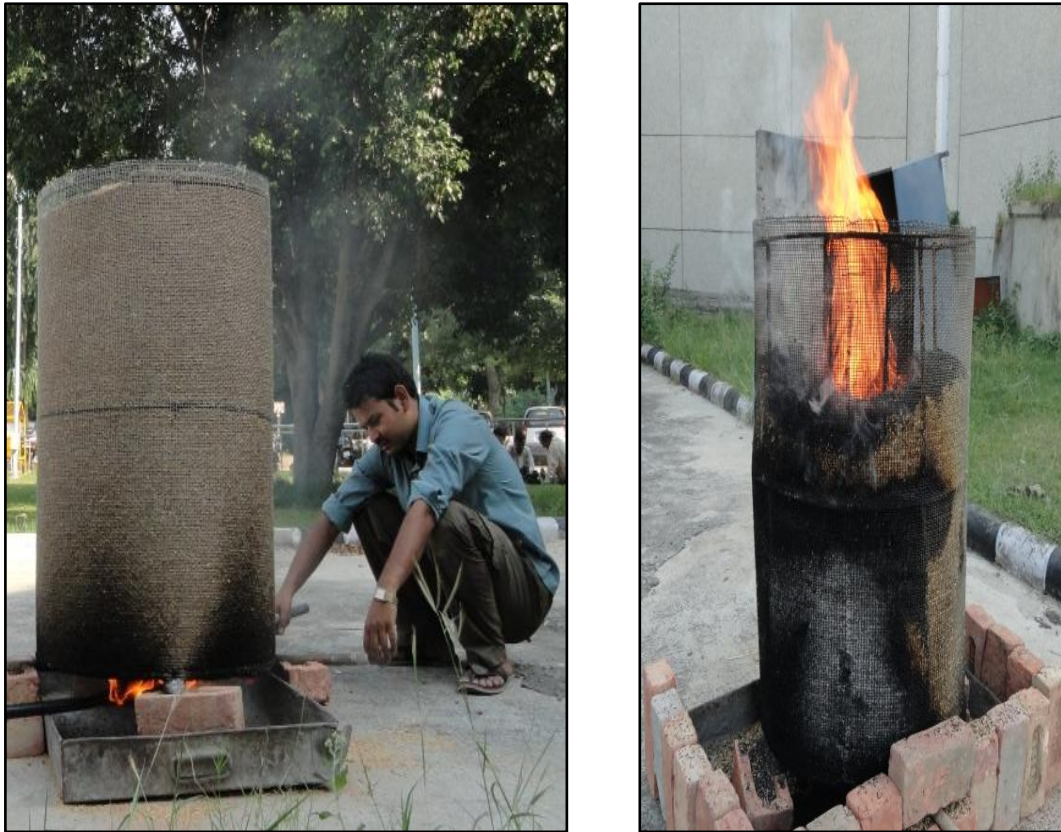
Figure 3.5 Burning the husk in the burner
