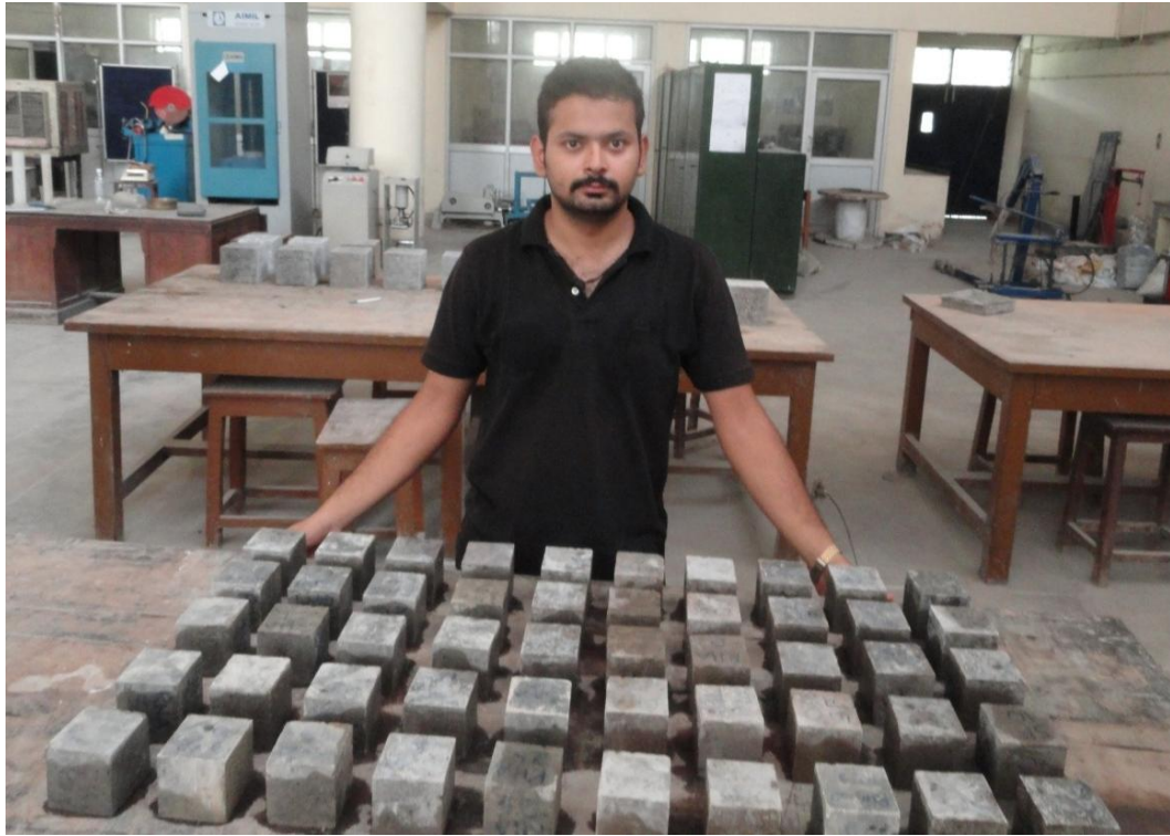
Figure 4.7: Photo of mortar cubes of 7, 28, 56, 90 days curing
