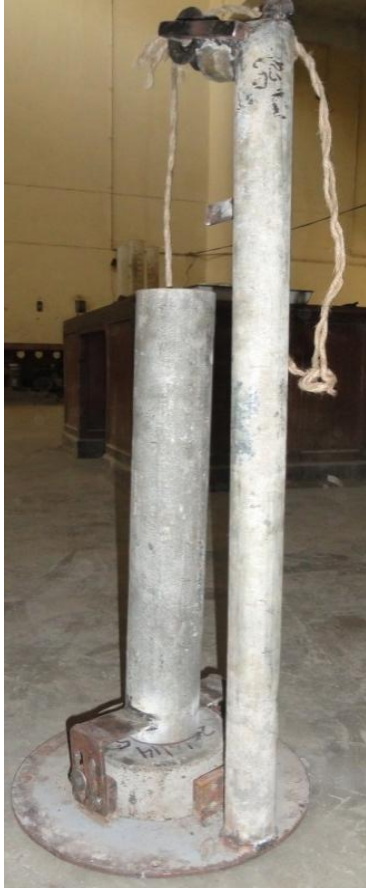
Figure 4.18: Impact test apparatus
