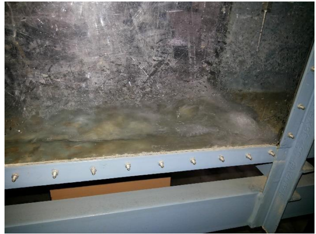
Figure 15: Hydraulic Jump from outside the flume
