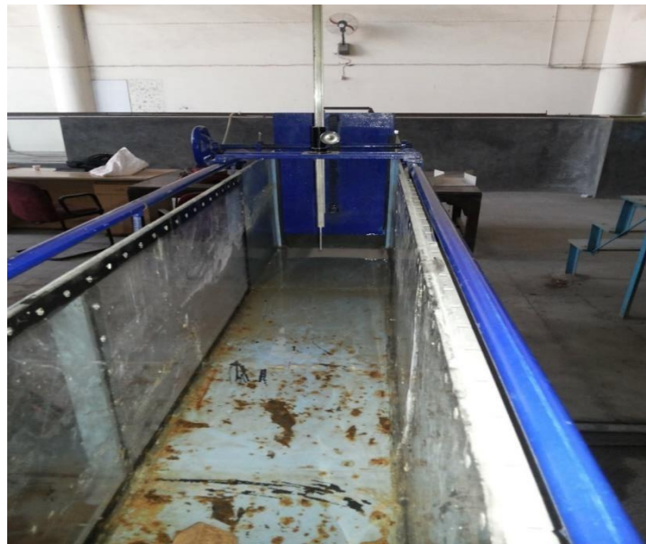
Figure 10: Point Gauge Fitted on the Flume
