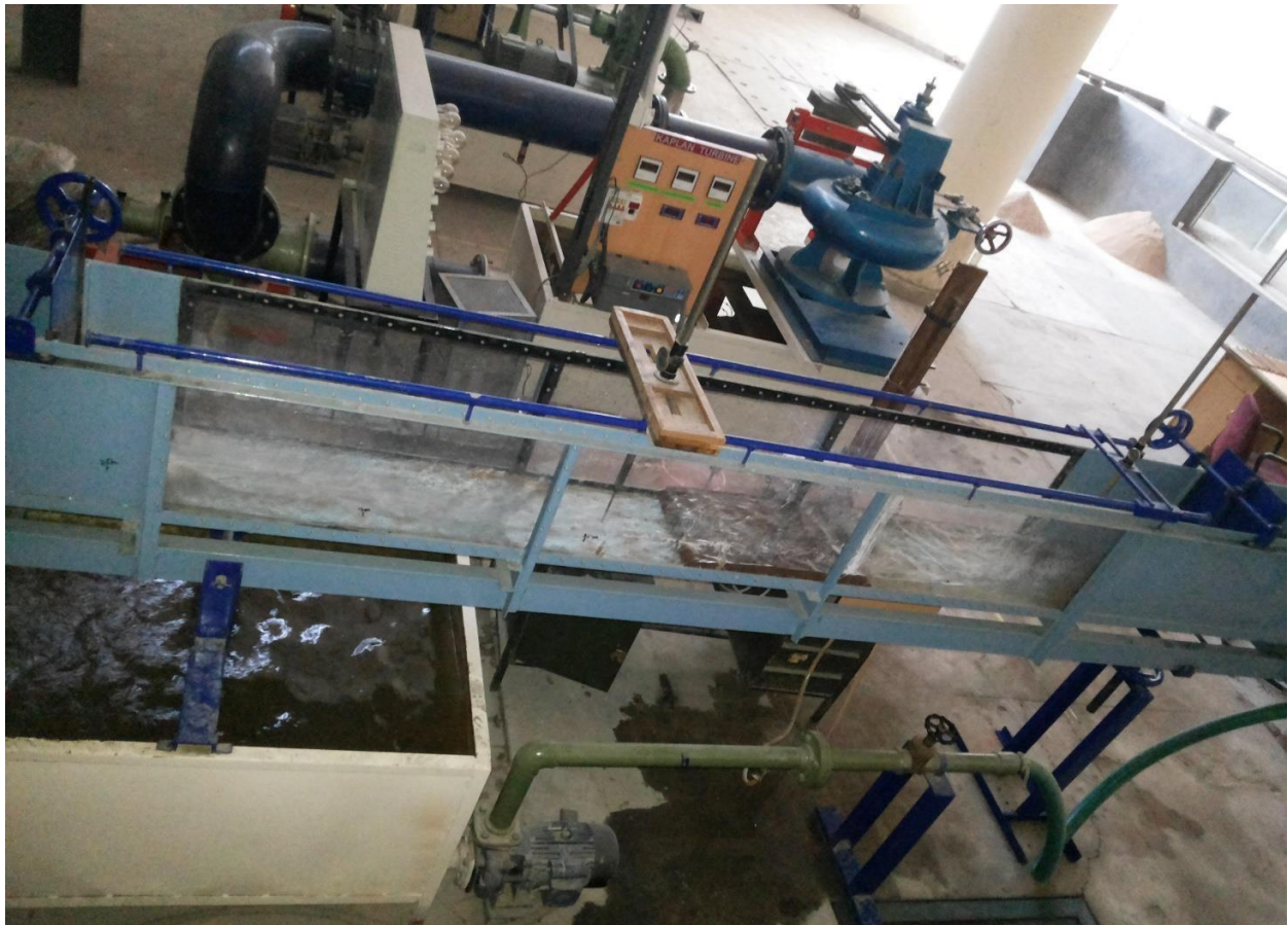
Figure 13: Flume Showing Hydraulic Jump
