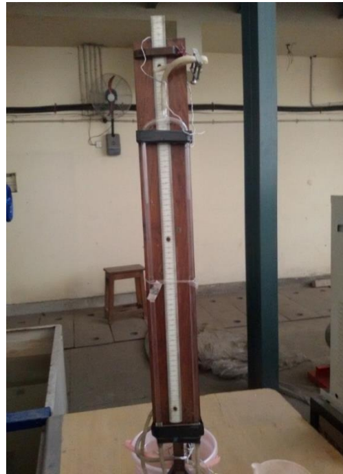
Figure 12: Pitot Static Tube Fitted with Manometer
