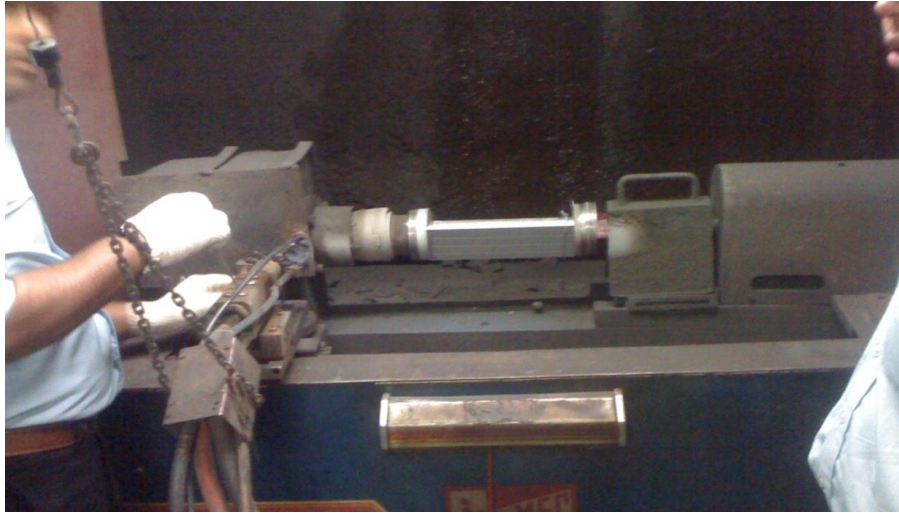
Fig. 4.2: Coating formation on the sample by air plasma arc spray machine
