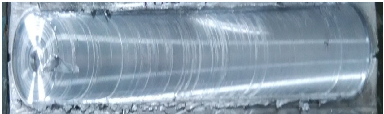
Fig.11. After processing plate (FSPed-Al/ZrB 2 5 %)
