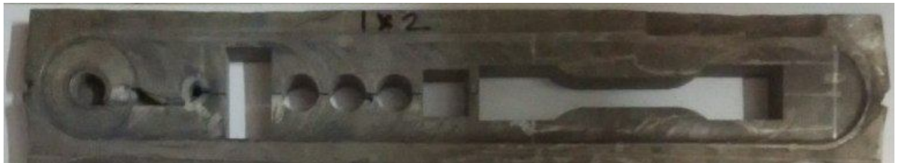
Fig.15. After wire cut through EDM - FSPed-Al/ZrB2 5%
