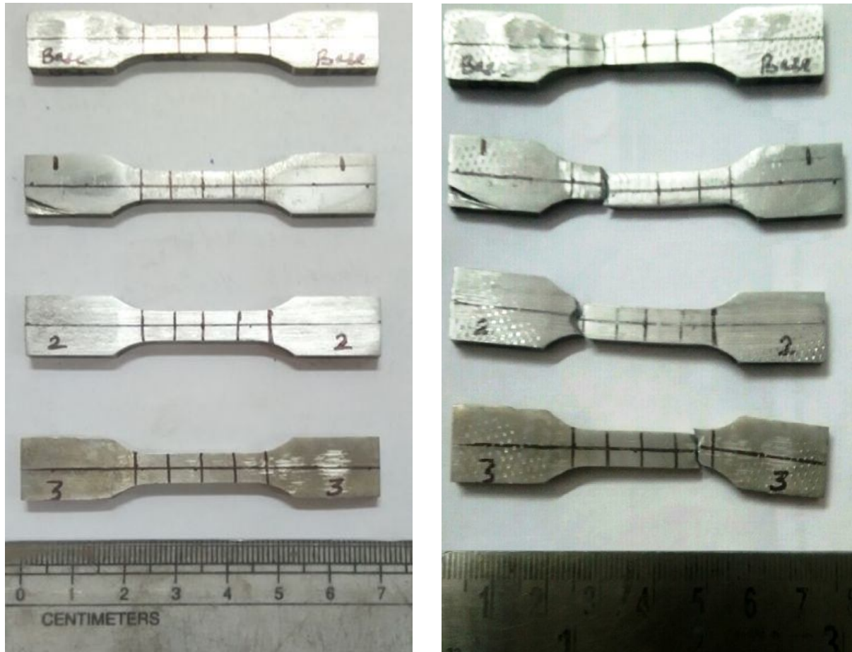
Fig.46. Tensile test before and after
