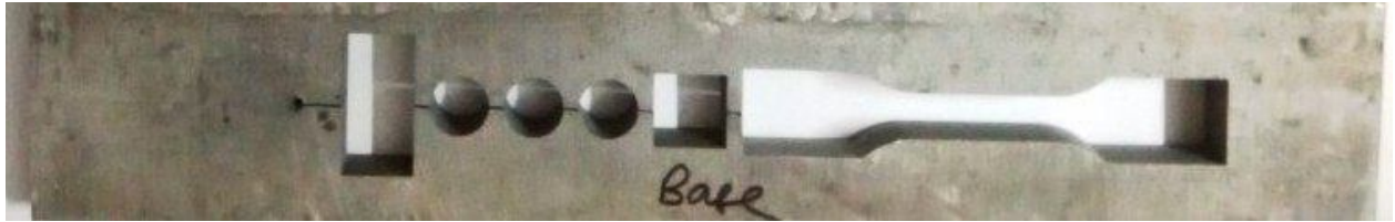
Fig.13. After wire cut through EDM-base
