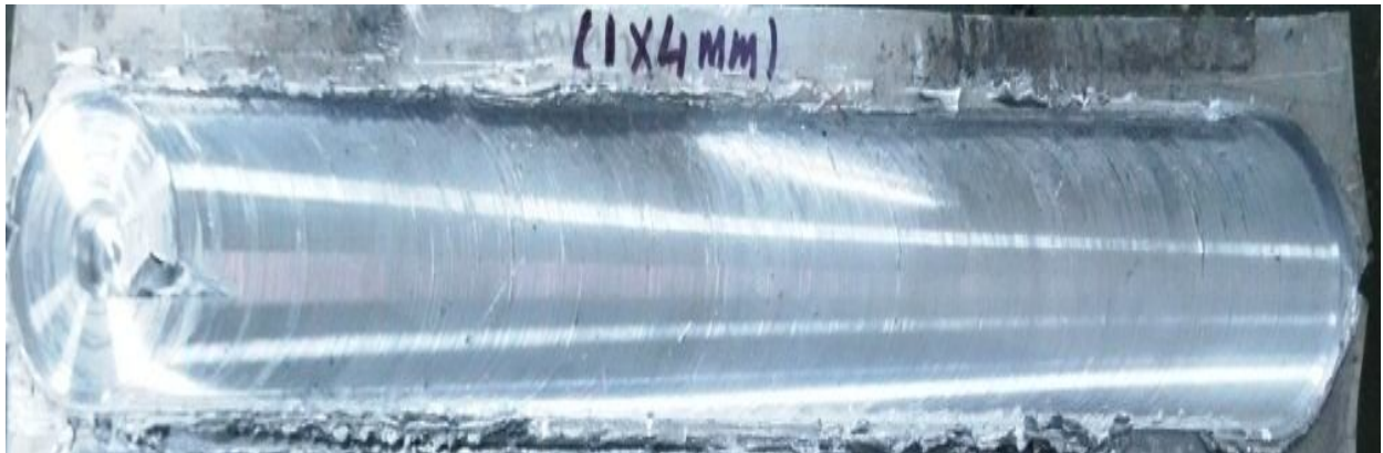
Fig.12. After processing plate (FSPed-Al/ZrB 2 10 %)
