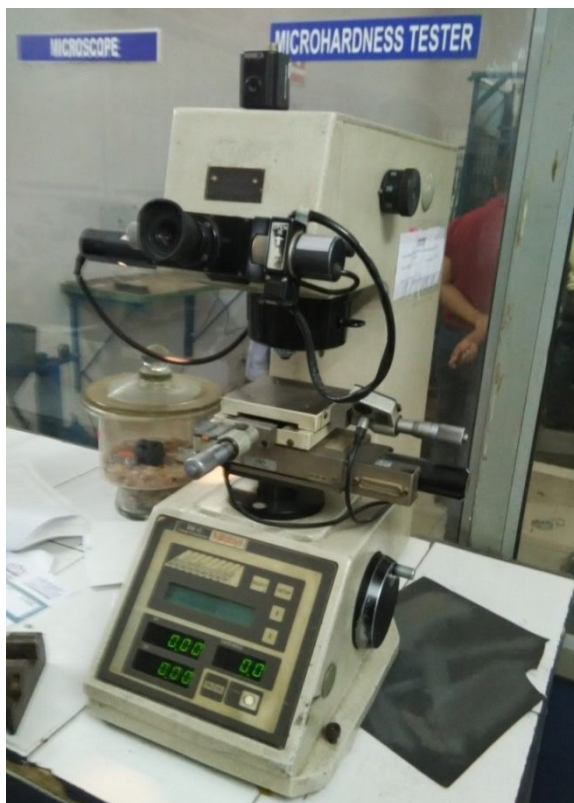
Fig.20. Vickers Hardness Testing Machine
