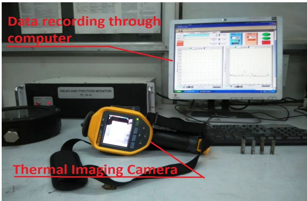
Fig.24. Computer and Thermal Imaging Camera for data recording
