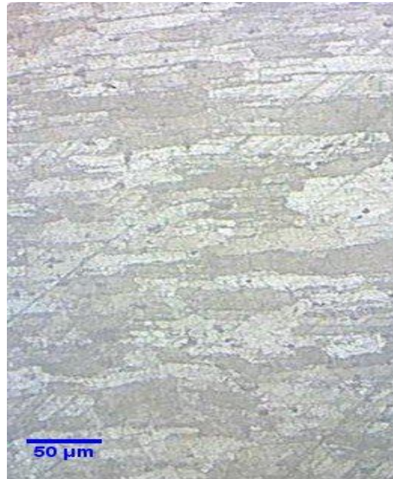
Fig.28. Microstructure of Base material Al7075/T651
