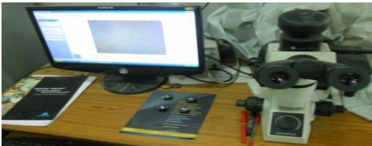
Fig.19. Optical Microscope setup for micro-structural observation
