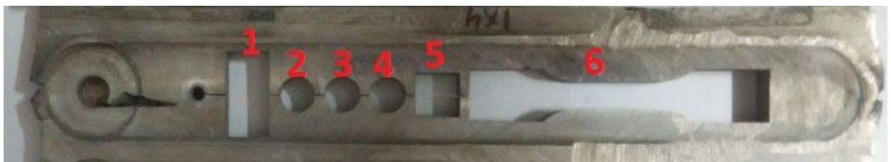
Fig.16. After wire cut through EDM - FSPed-Al/ZrB2 10%
