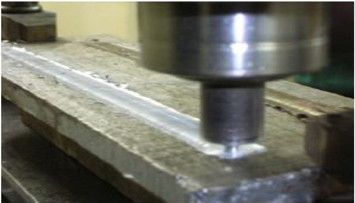
Fig.2.FSP of a plate
