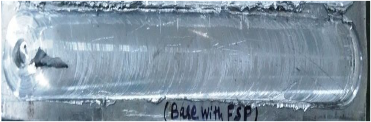
Fig.10. After processing plate (FSPed-Al/ZrB 2 0 %)
