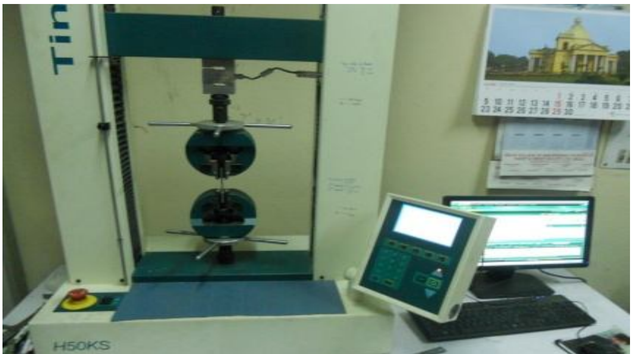
Fig.27. Computerized Tensile Testing Machine
