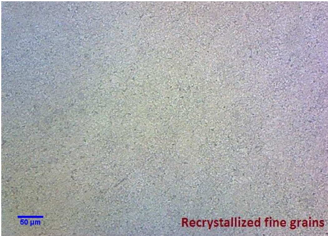
Fig.32. Microstructure (Nugget Zone) FSPed -(Al/ZrB2 0%)
