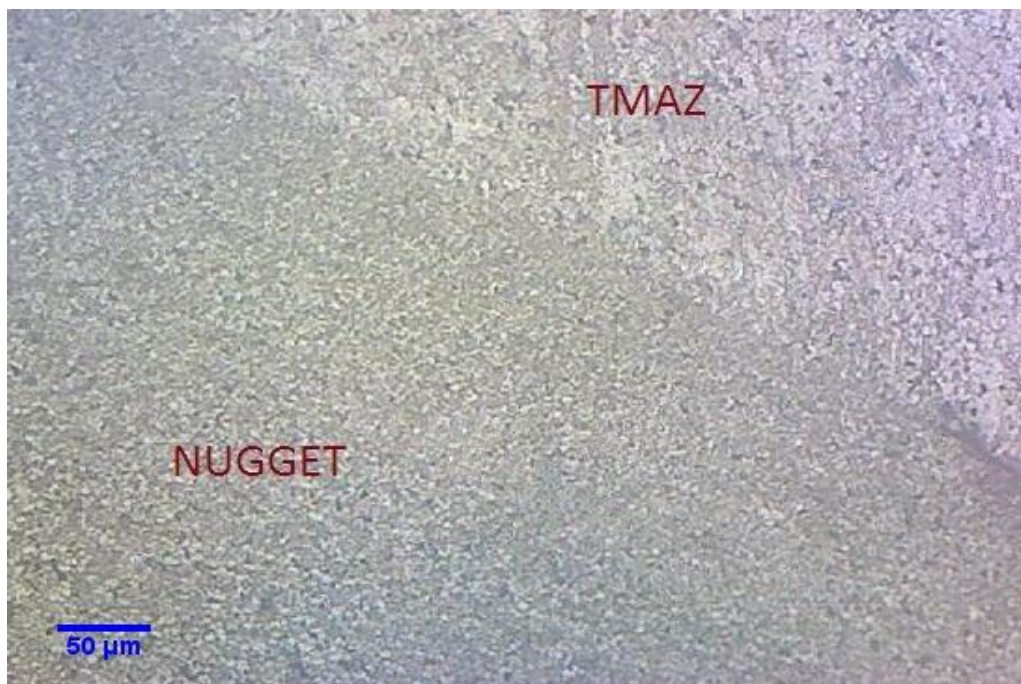
Fig.29. Microstructure - FSPed without particles (Al/ZrB2 0%)
