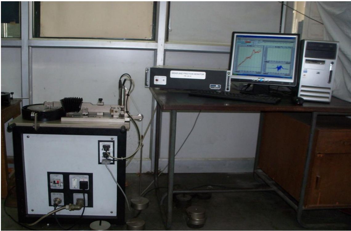
Fig 4: Pin on Disc type Tribometer Friction & Wear Machine set up
