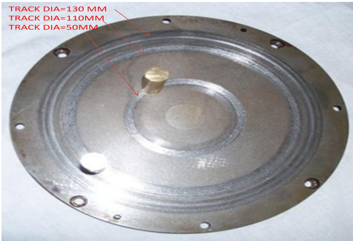
Fig 6 : DISC WITH DIFFERENT TRACK DIAMETER
