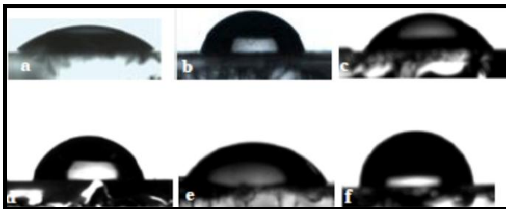
Fig. 6.3: Contact angle measurement images of (a) ITO coated glass plate; (b) APTES/ITO-glass; (c)GO/APTES/ITO-glass; (d) RGO/APTES/ITO-glass; (e) ZnS(MPA)-RGO/APTES/ITO-glass; (f) Ab-cMb/ZnS(MPA)-RGO/APTES /ITO-glass
