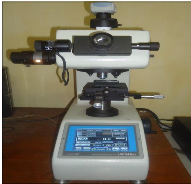
Fig. 10: Micro indentation hardness tester
