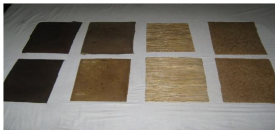
Fig 8: Bio-composite sheet with different types of fibres
