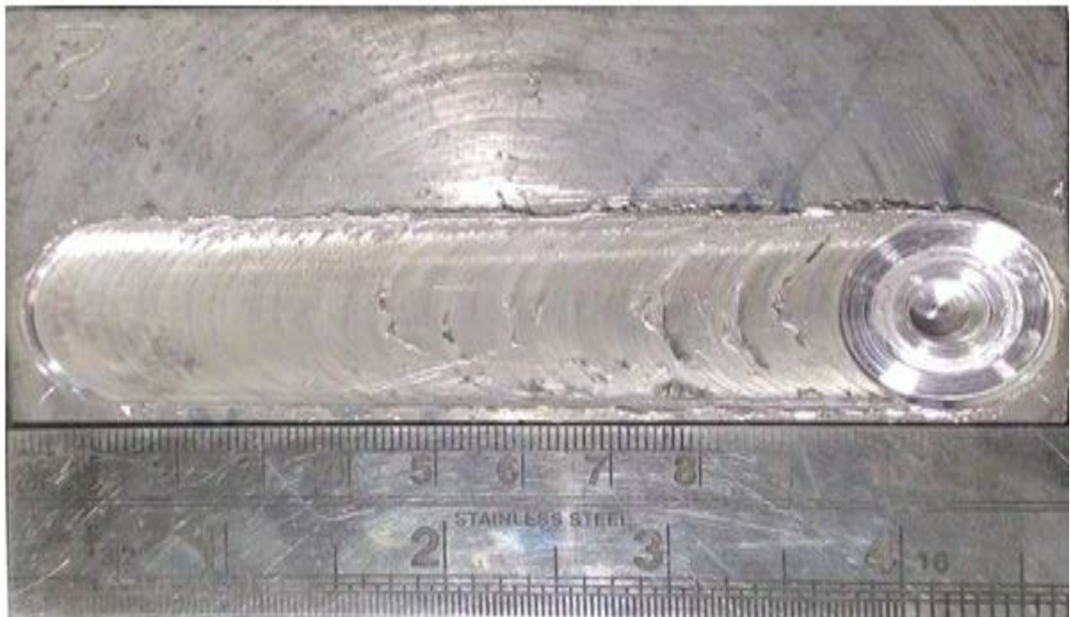
Figure 3.5 Surface appearance of FSPed H1 alloy plate without B 4 C.
