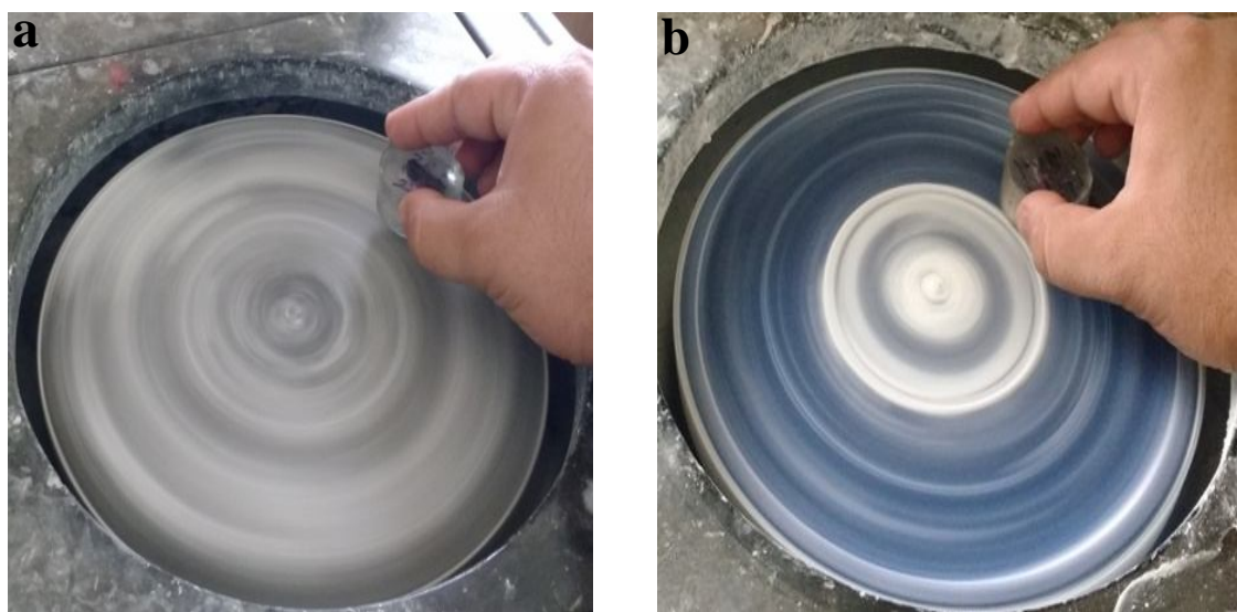
Figure 3.10 Wet Polishing by (a) Fine grit emery paper (b) Alumina Powder
