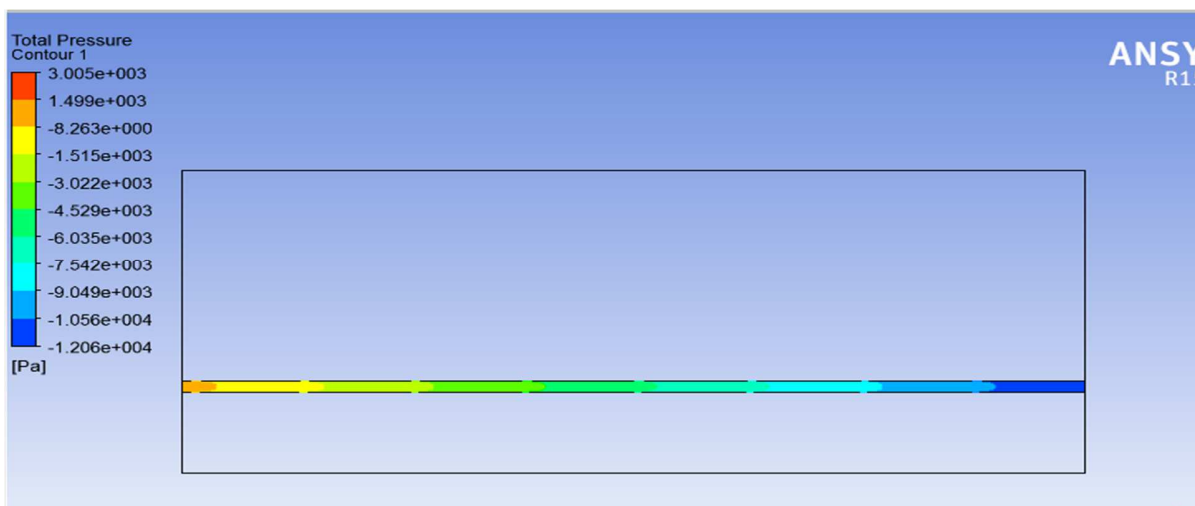
Figure 5.19: Pressure contours for water along the channel at Re=600
