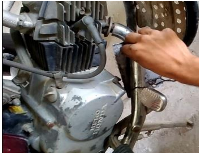
Figure 4.4- TEG located on exhaust pipe of vehicle
