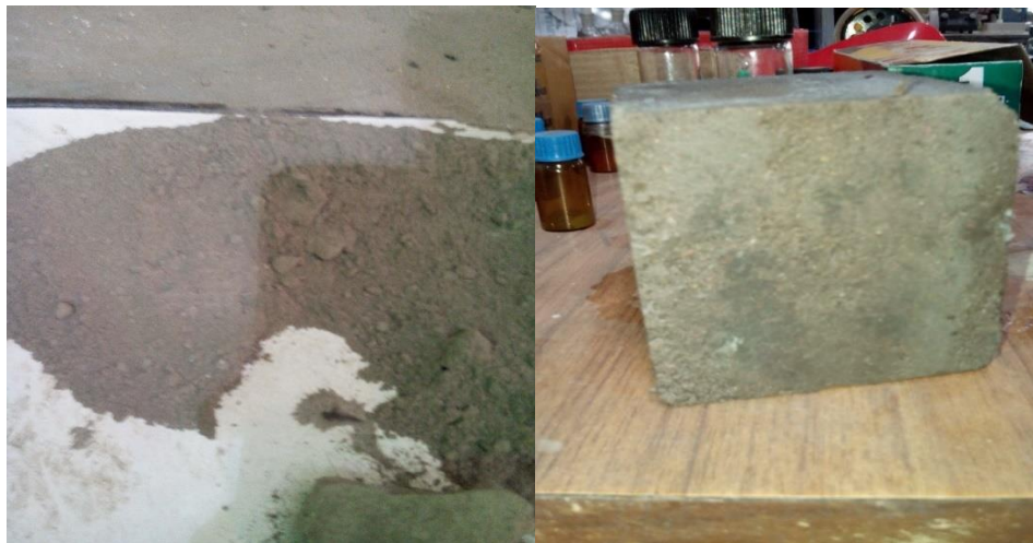
Fig.7(a) Cement mixed with PET and (b) Brick formed of PET and cement
