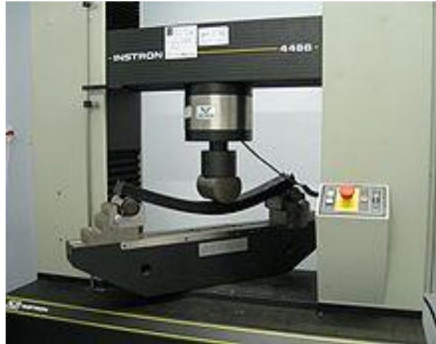
Fig.3 Test fixture on universal testing machine for three-point flex test
