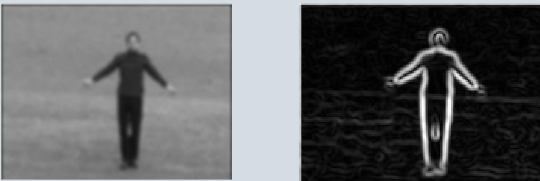
Figure 2.6: The gradient magnitudes in the smoothed image as well as their directions are determined by applying the Sobel-operator
