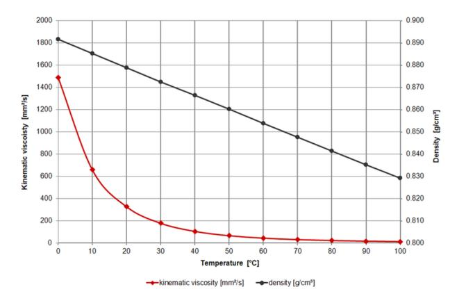
RESULT: kinematic viscosity is as depicted above for different temperatures
