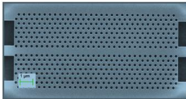
Figure 2.7: Fabricated photonic crystal W1 waveguide and input/output strip waveguides, formed by a single line defect
