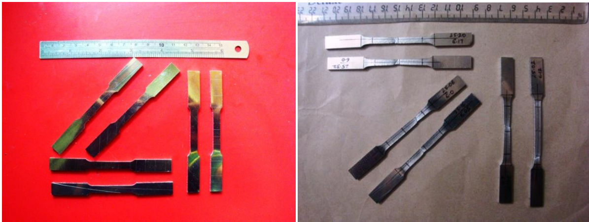
Fig. 4.4 Tensile specimens at different orientations (Before And After the test)
