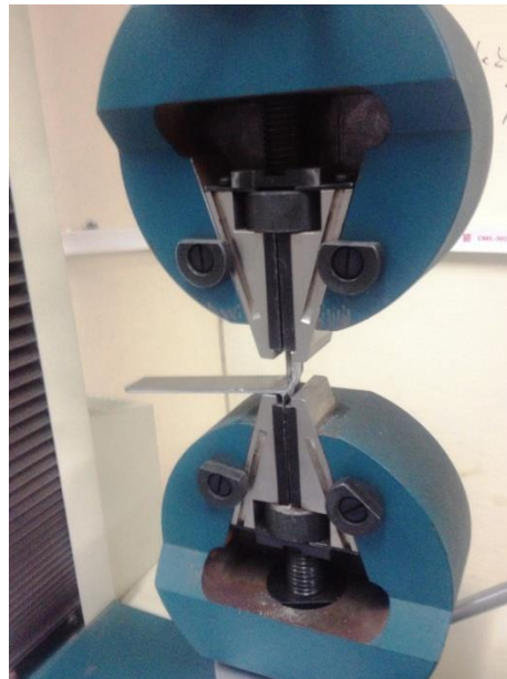
Fig. 4.1 Peel test arrangement on 50kN UTM
