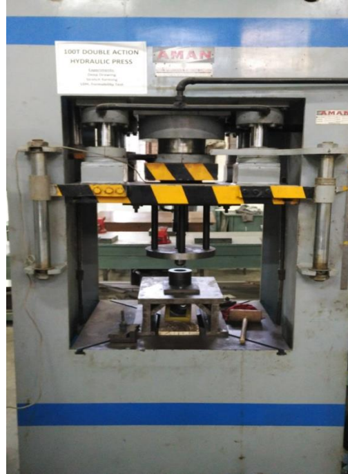
Fig. 4.10 Experimental setup on 100-tonne Hydraulic press
