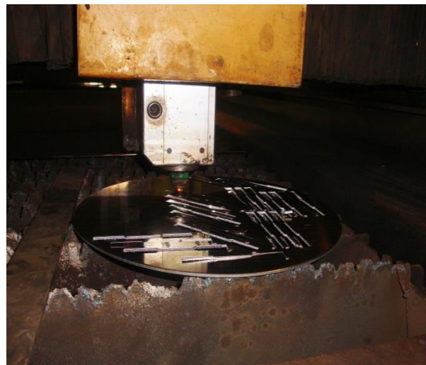
Fig. 4.3 Laser cutting of tensile specimens
