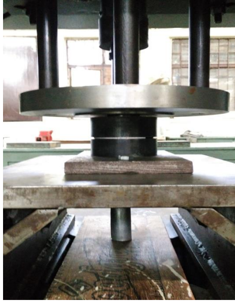
Fig. 4.11 Arrangement of Die-Holder-Punch-Blank on hydraulic Press bed
