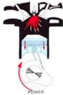
Fig 1.1(c) Power Stroke
