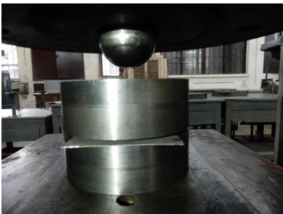
Figure 24: Stretch forming experimental setup
