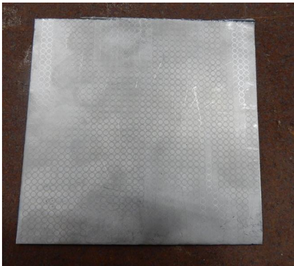
Figure 22: Grid of circles marked on the specimen sheet
