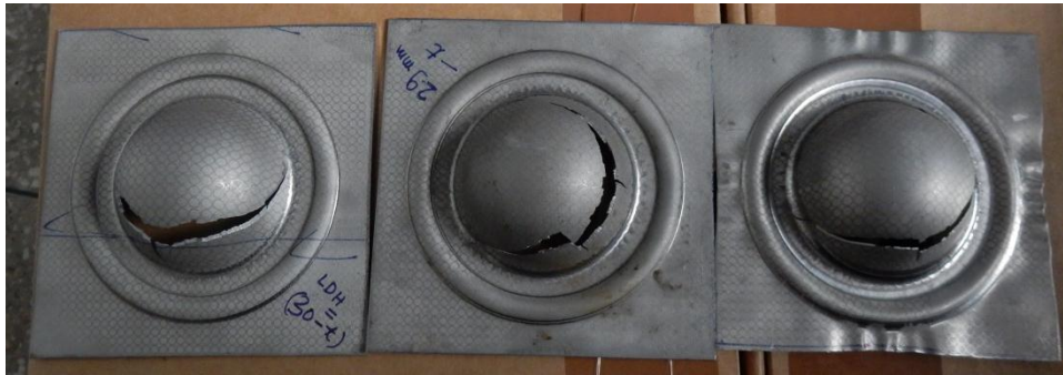
Figure 25: Specimens cracked during the experiments
