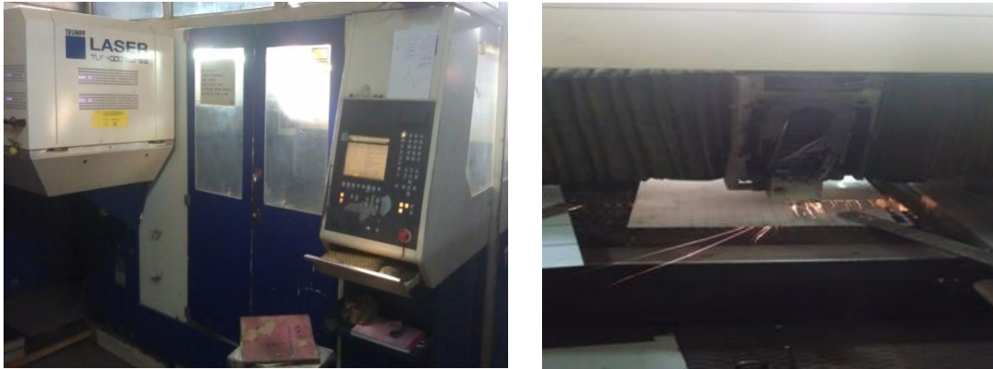
Figure 14: Specimen cutting using Lazer machine
