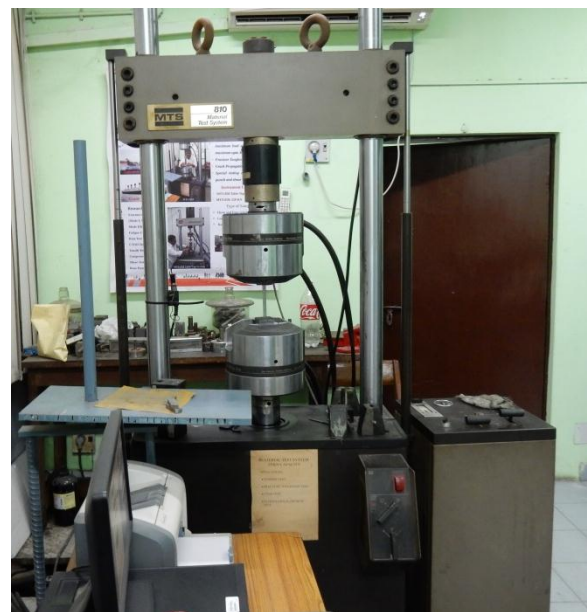
Figure 11: MTS, 800 m/c in NDR lab at IITD
