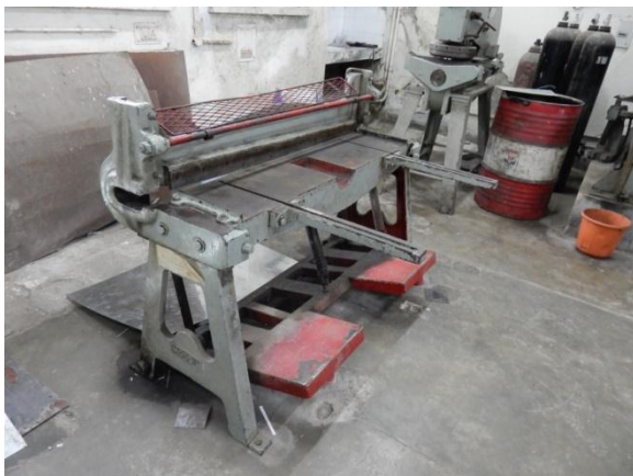
Figure 23: Shearing m/c used and photo of specimens
