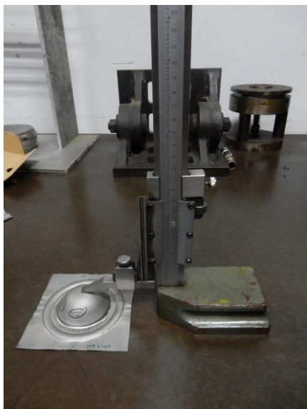
Figure 28: Dome height measurement using vernier height gauge
