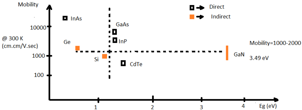
Fig. 2.5: Relative energy band diagram and mobility of different material.
