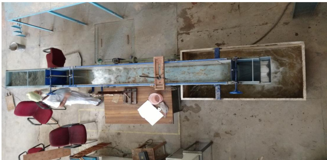
Fig. 3.3 Hydraulic Flume (Top view)
