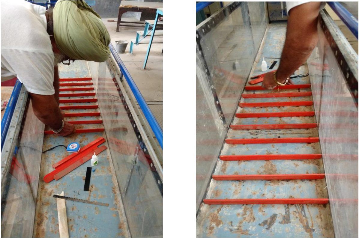
Fig. 3.2 Fixing of rectangular block
