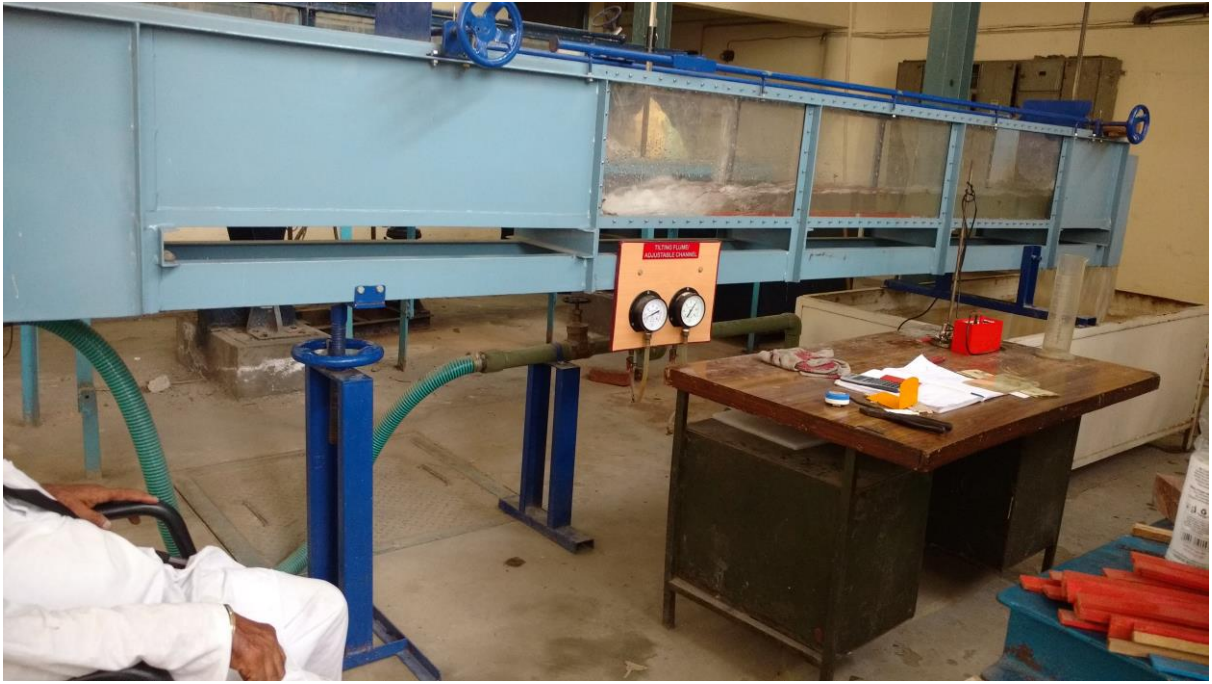
Fig. 3.13 Hydraulic flume experimental setup and jump formation
