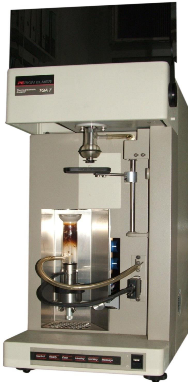
Fig. 4.9: Picture of Thermo gravimetric Analysis (TGA) instrument
