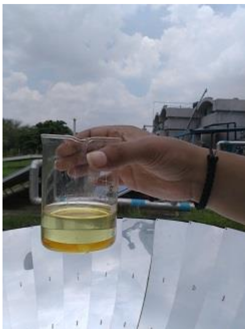
Figure 5.6- Crude biodiesel produced after transesterification at medium scale
