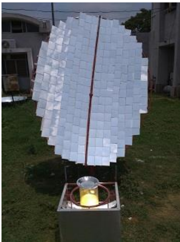
Figure 5.5- Transesterification process using Scheffler reflector
