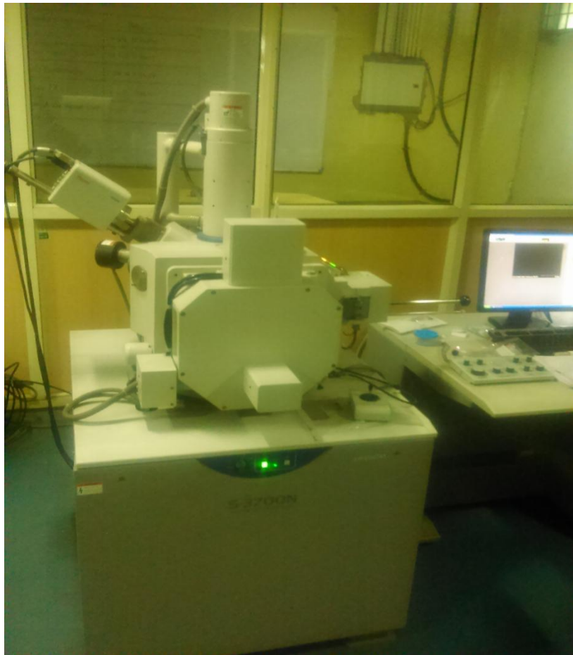
Fig-13-SEM HITACHI, model no. S-3700N with EDX with X-ray at DTU, Delhi
