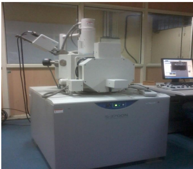
Figure 21: SEM HITACHI, model no.S-3700N with EDS-X with X-ray at DTU, Delhi
