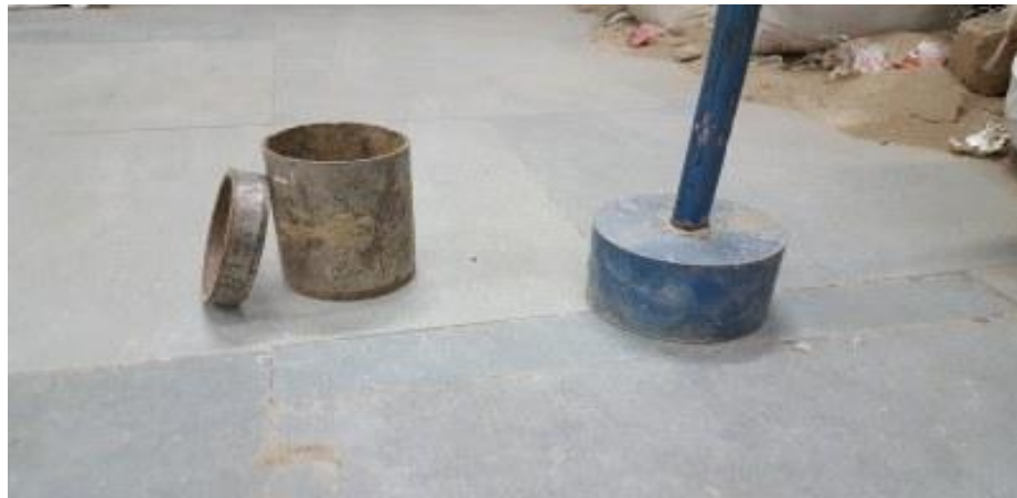
Figure 5.1 Core cutter and rammer for bulk density measurement
