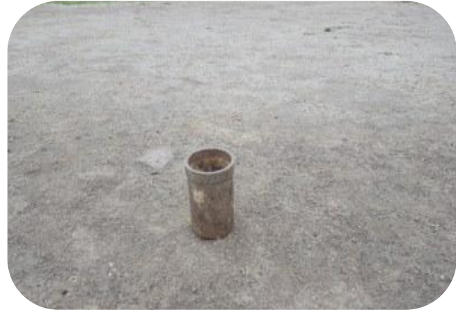
Figure 5.4 b) Bulk density measurement at site S3
