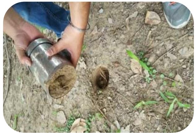
Figure 5.8 b) Bulk density measurement at site S7
