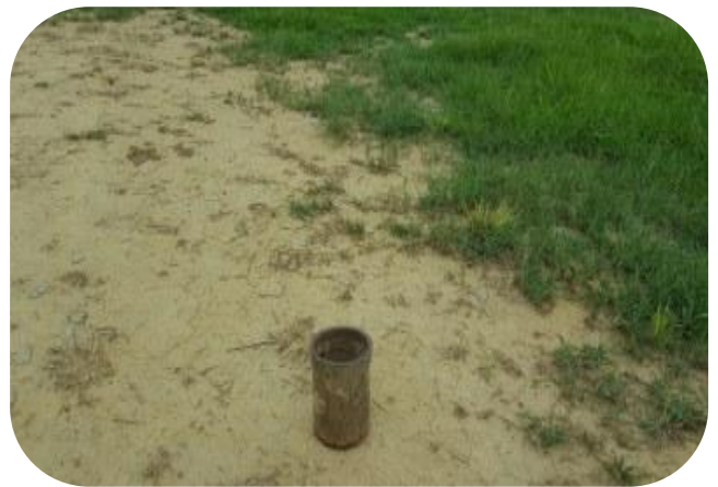
Figure 5.3 b) Bulk density measurement at site S2
