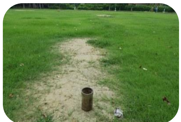
Figure 5.9 b) Bulk density measurement at site S8
