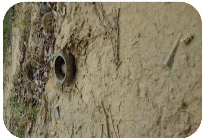
Figure 5.5 b) Bulk density measurement at site S4
