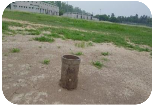
Figure 5.2 b) Bulk density measurement at site S1
