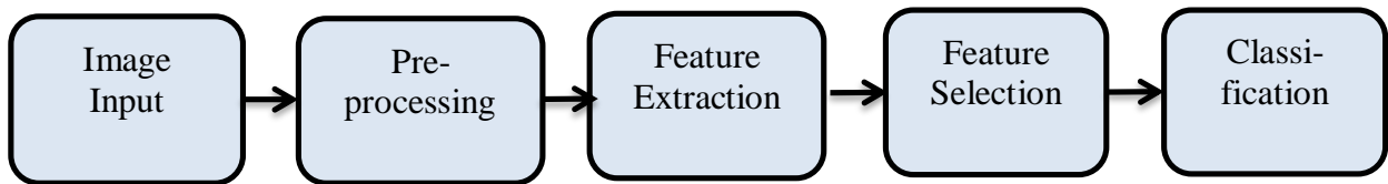
Figure 1.1 Flow diagram of Hand gesture recognition system
