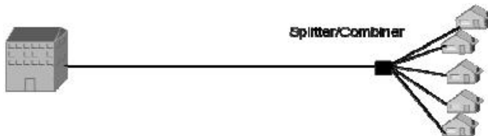
Fig. 2.3 Passive Optical Network architecture
