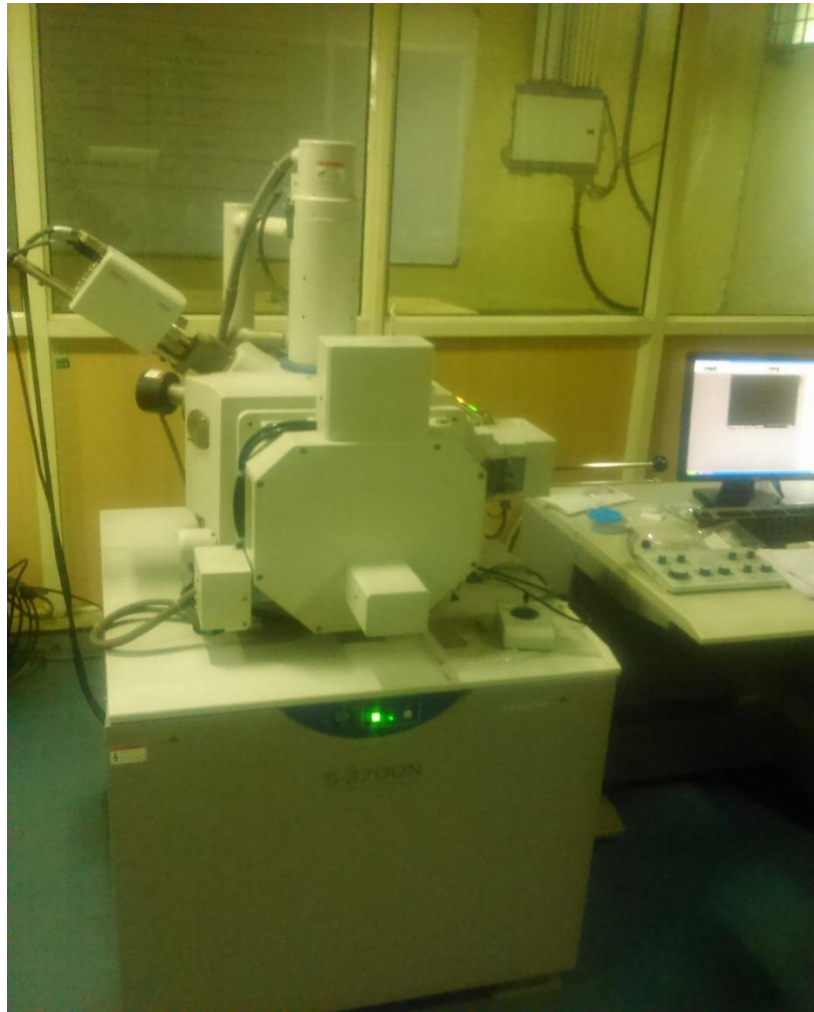
Figure 2.1: A pictorial view of SEM HITACHI, model no. S-3700N with EDX with X-ray
