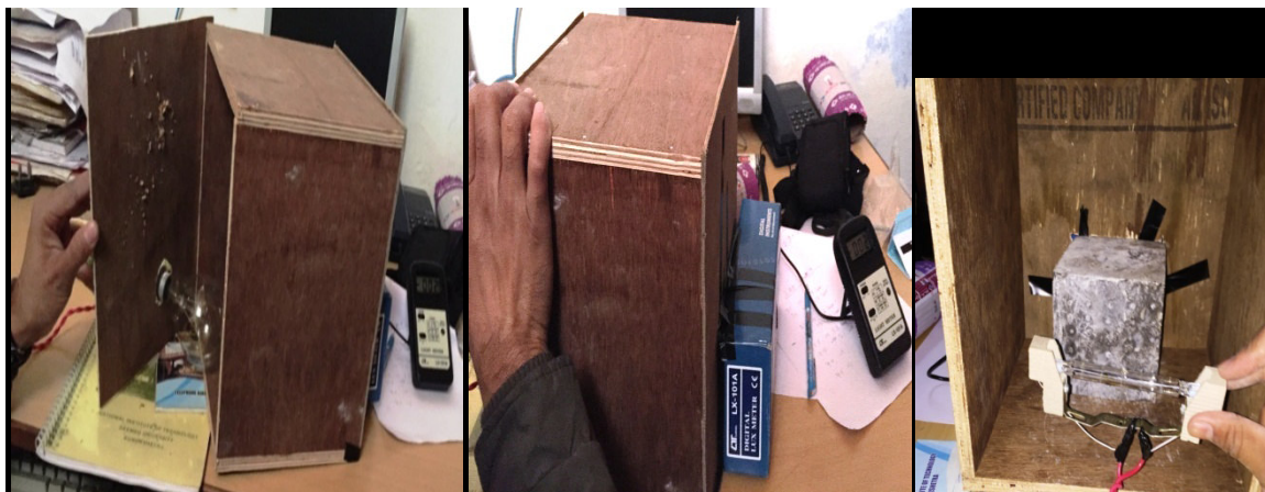
Fig 3.8: Experimental setup to find light guiding property of light transmitting concrete
