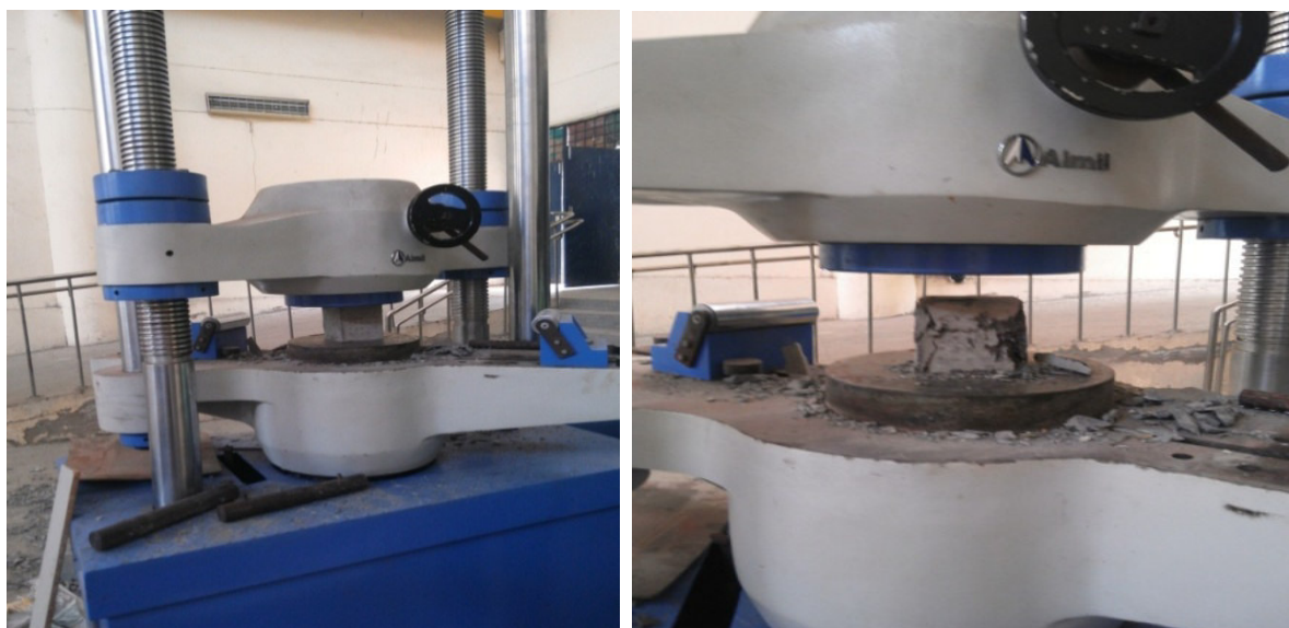
Fig3.9: Compressive strength test setup showing light transmitting concrete cube.
