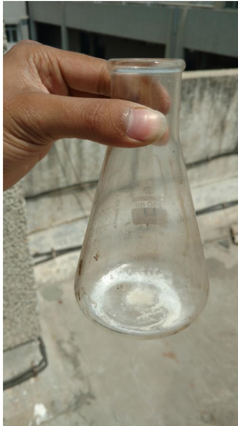
Figure 3.4. Sediment sample after acid digestion
