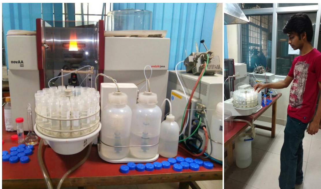
Figure 3.7. Heavy Metal Analysis on AAS
