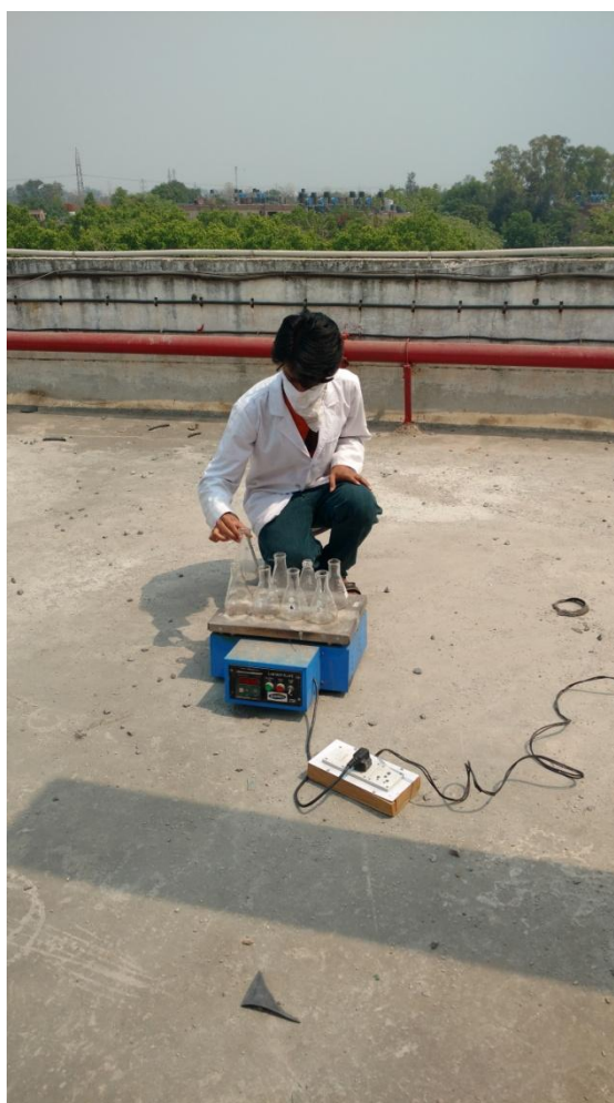
Figure 3.3. Acid Digestion of Sediments on Hot Plate
