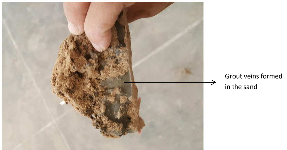
Figure 4.9. Grout Veins Formed in the Sand
