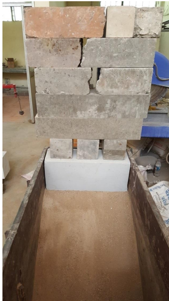
Figure 4.6. Loading Applied on the Embankment
