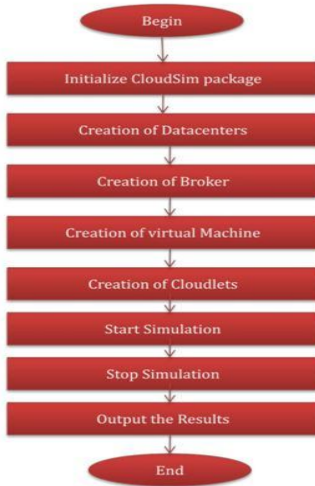
Figure 6.3: Flow of program execution in CloudSim
