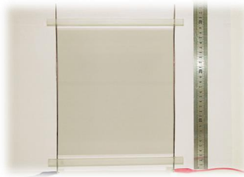
Figure 1.10 Thin film, flexible, transparent, magnet-free, and stretchable nanotube speakers.
