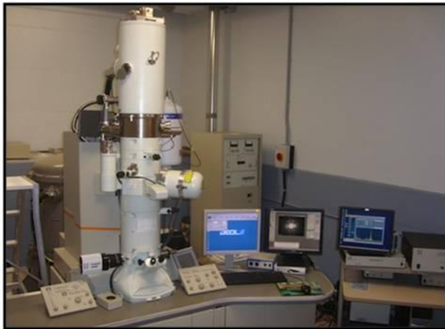
Figure 4.1 Transmission electron microscopy (TEM): Hitachi Model, H-800 TEM
