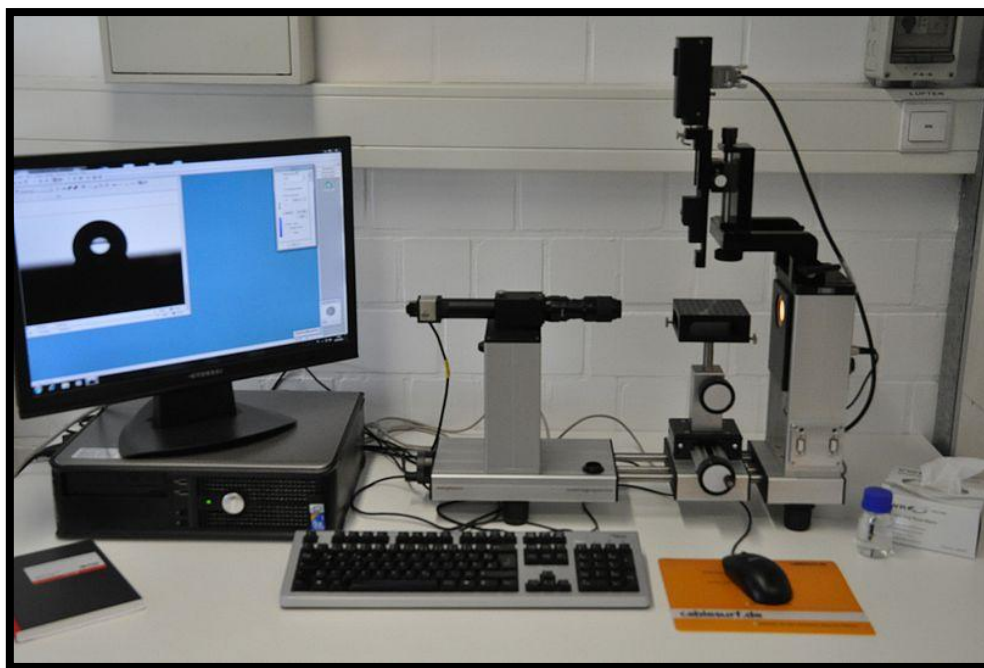
Figure 4.3 Optical Contact angle (OCA) instrument model of Data Physics; model number OCA15EC.
