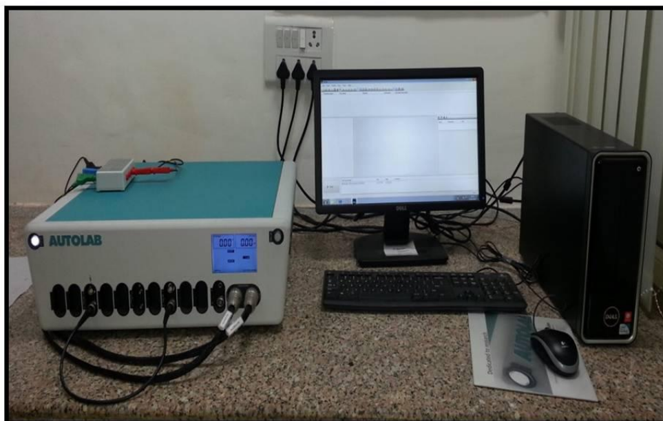
Figure 4.4 Potentiostat/Galvanostat instrument: Metrohm Autolab
