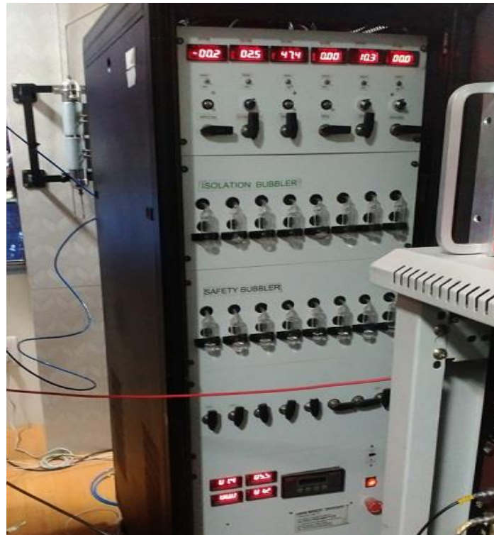
Fig 2.10 Front Panel of Gas Mixing Unit
