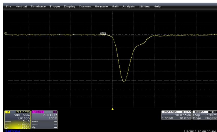
Fig 4.1 Low Amplitude RPC pulse
