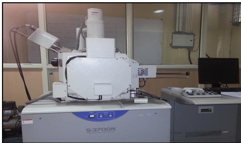
Figure 4.2: Scanning electron microscope (SEM) Instrument.
