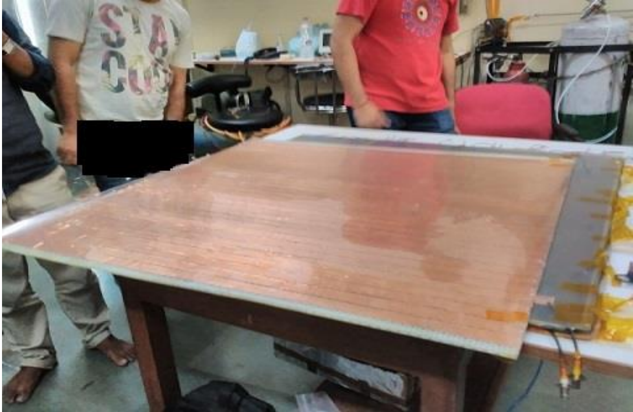
Fig 3.7 Assembling of 100 m X 100 m RPC.
