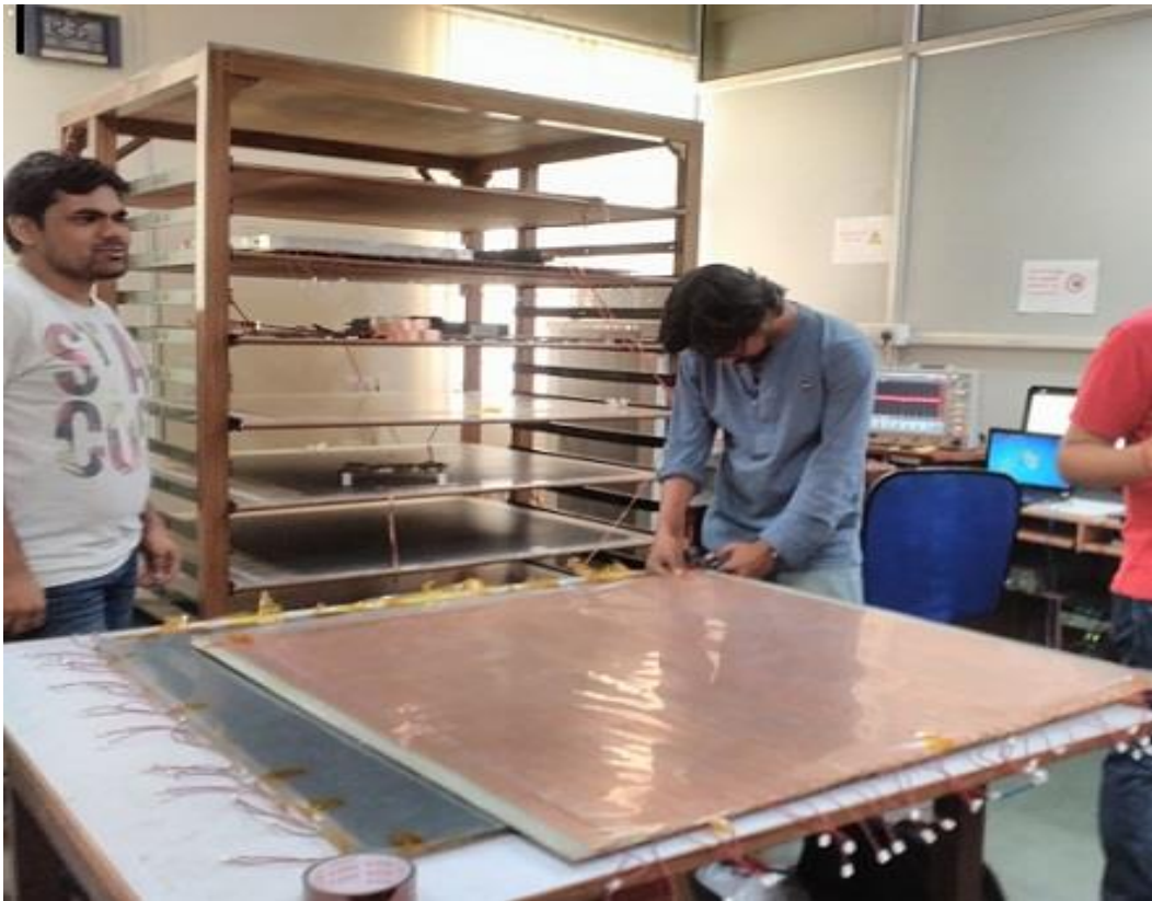
Fig 3.3 Fabrication of Pickup Panel for interfacing with front-end electronic
