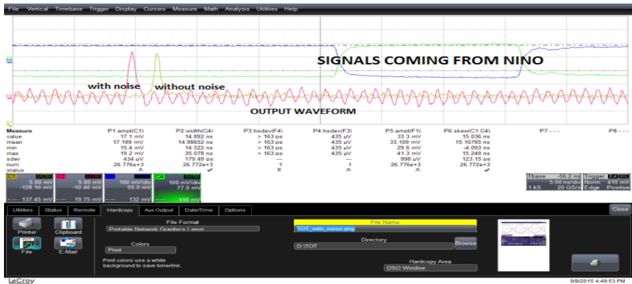
Fig 4.7 The different signals investigated: the primary signal without noise (yellow), the primary signal with noise (red) and the signals coming from the NINO amplifier (green and blue).
