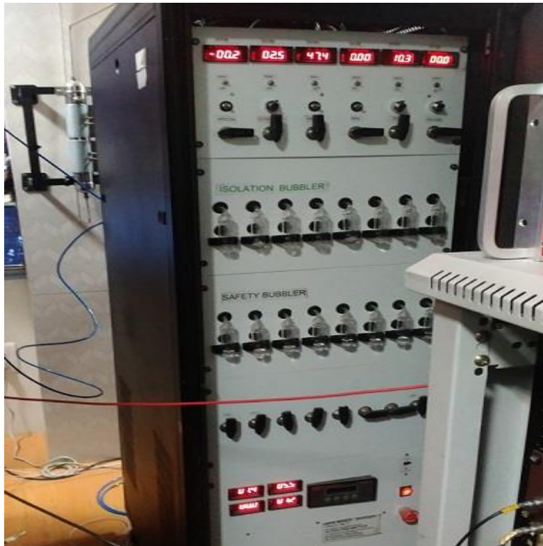
Fig 2.7 Gas Mixing Unit
