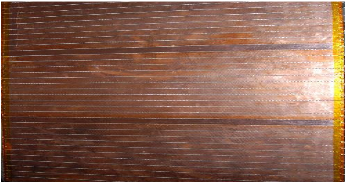
Fig 3.6 Honeycomb panel with milled copper pickup strips
