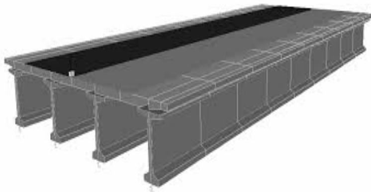
Figure 3.7 I - Girder (Precast) with Cast-In-Situ Slab
