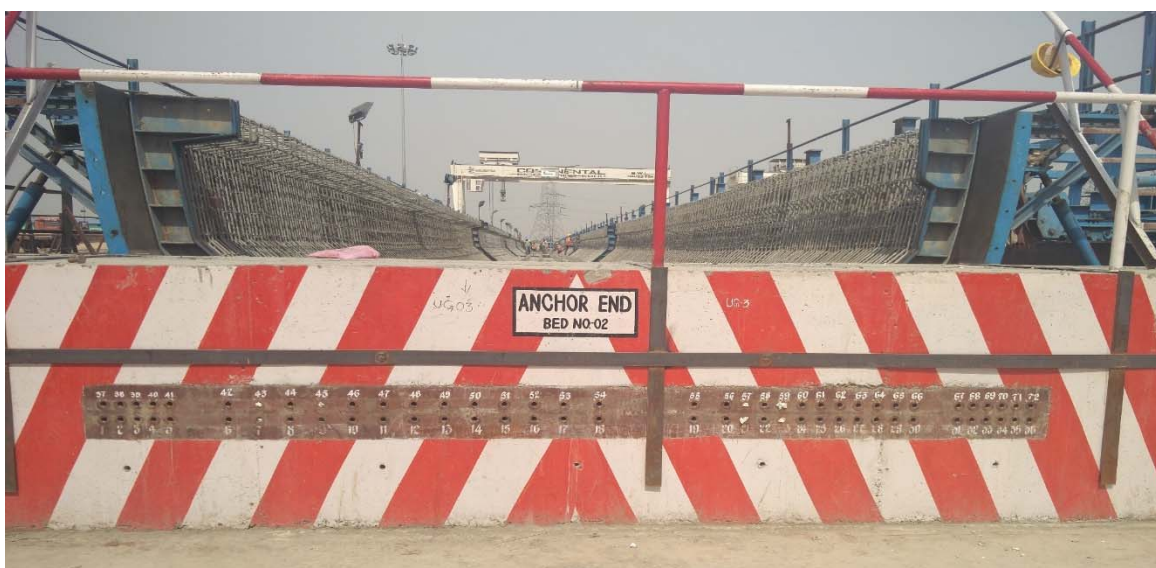
Figure 3.13 A Typical Anchor End
