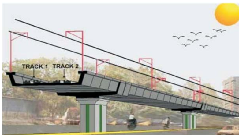
Figure 3.8 U - Girders supporting 2 Tracks – Precast Segmental
