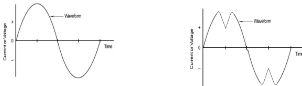
Fig 5.3: (a) Ideal Sine wave (b) Distorted Waveform
