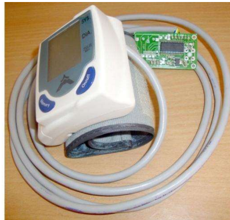
Figure 4.3 BP sensor with ARDUINO operability and serial communication.
