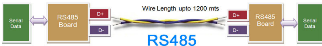
Fig 2.4 RS485 2 wire connection
