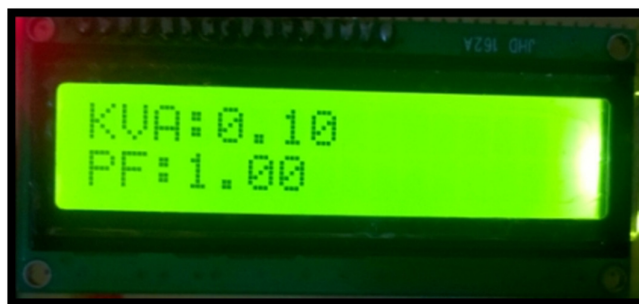
Figure 3.10(c) Apparent power and phase measurement
