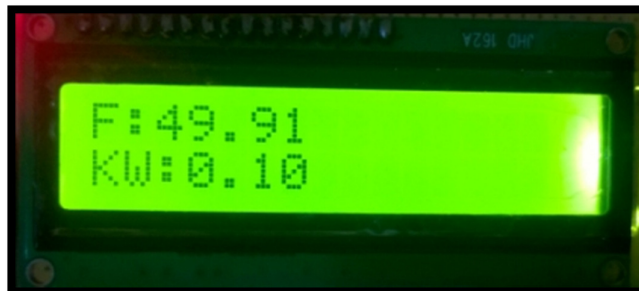
Figure 3.10(b) Frequency and real power measurement
