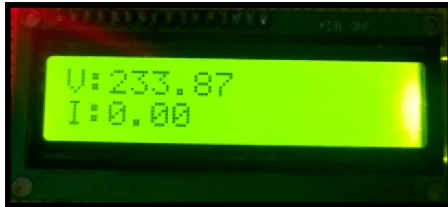
Figure 3.8(a) Voltage and Current measurement
