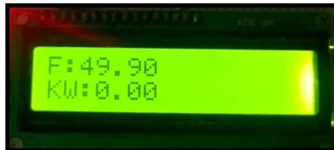
Figure 3.8(b) Frequency and Real Power measurement
